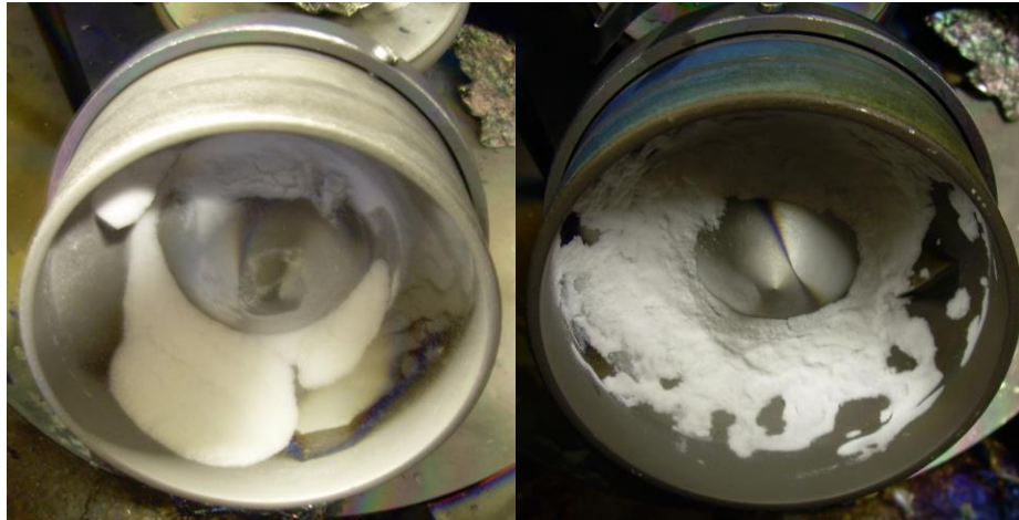
Figure 4.19: a) Spheres (8ml) 50 \mu\text{m} sieved ( >50 \mu\text{m} ) are still trickling after 1h rotating in the coating vessel at 1.5 Pa argon; most of the spheres are at the bottom of the coating vessel, which indicates good trickling behaviour; b) spheres (8 ml) 50 \mu\text{m} sieved ( <50 \mu\text{m} ) stick to one another and to the surface quite instantly; the image shows the spheres after 15min rotating in the coating vessel at 1.5 Pa argon; the stuck spheres are evenly distributed in the coating vessel.
