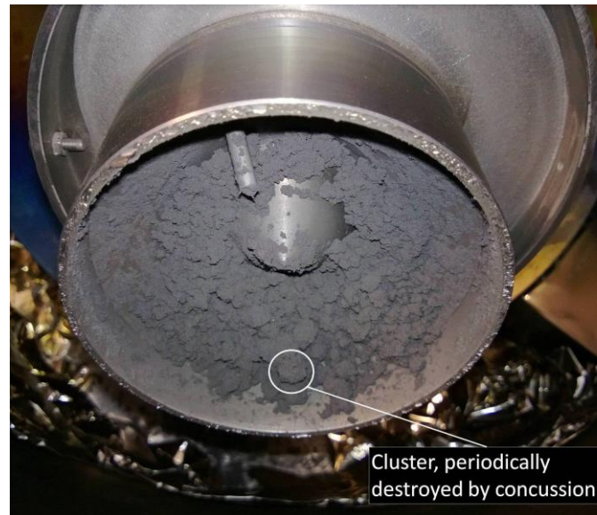
Figure 4.20: One hour titanium coated spheres directly after opening the vacuum chamber. The remaining clusters of coated glass micro spheres which form and break apart continuously during the whole coating process can still be seen. Most of the spheres are at the bottom of the coating vessel, which indicates good trickling behaviour.
