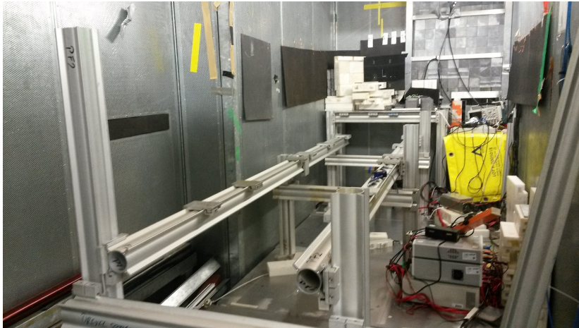
Figure 11: Aluminium table to carry the MONOPOL-experiment
