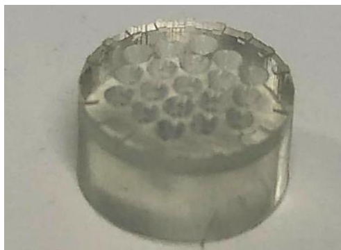
Figure 20. 3D printed Transfreez cryotube insert
