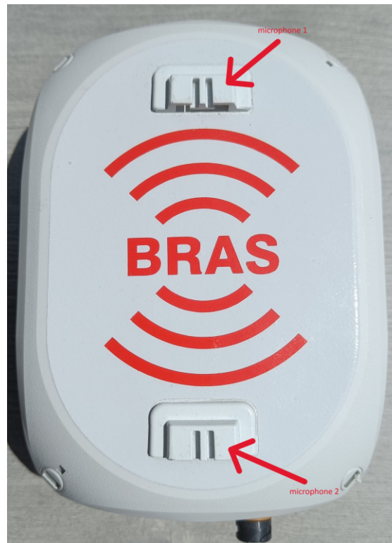
Figure 4.2: Sensorbox topview with microphone shields marked
