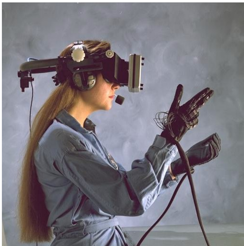
Figure 2.2: The data glove by Lanier [81]
