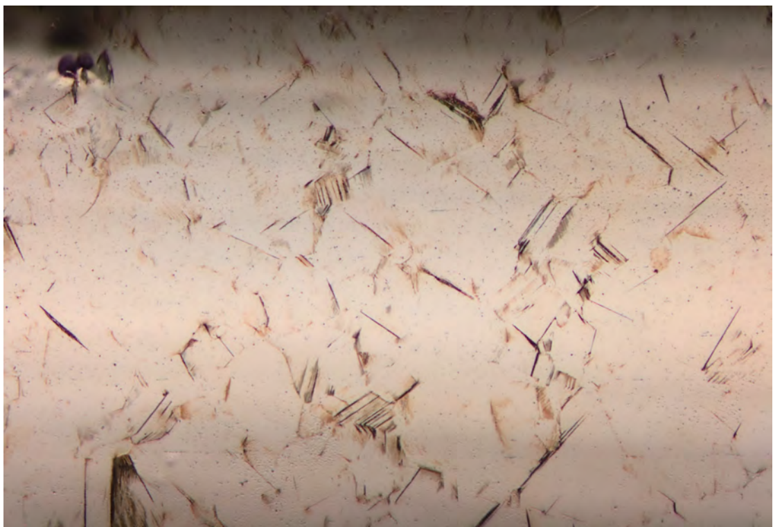
FIGURE E.13: Specimen U21 after N = 8.10 \cdot 10^5 cycles.
