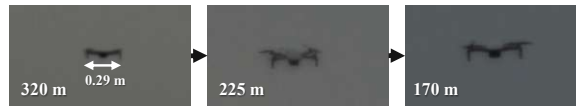
Fig. 8. Example image sequence depicting a UAV flying at up to 15 m/s towards the telescope system, while the automatic focus keeps the UAV in focus.
