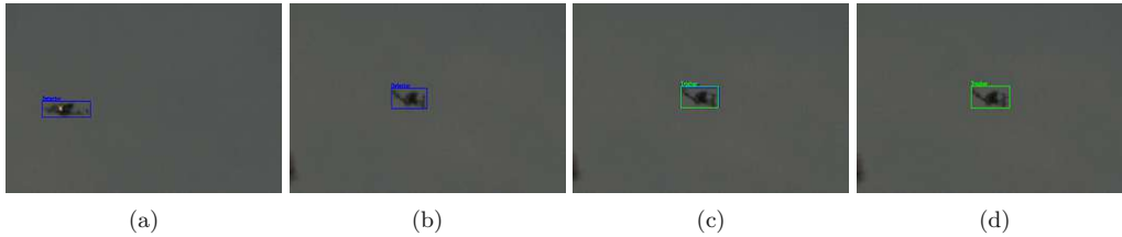
Figure 4: Image sequence of a detection and track of a UAV. The blue and green bounding boxes indicate the detector the tracker output.
