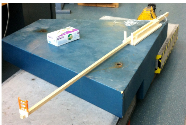
Figure 12.11: Sample holder used for irradiations in the horizontal beam tube
