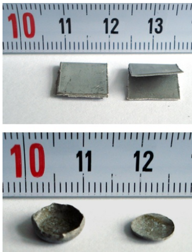
Figure 12.9: Cadmium covers folded and made into small cups to enclose the foil
