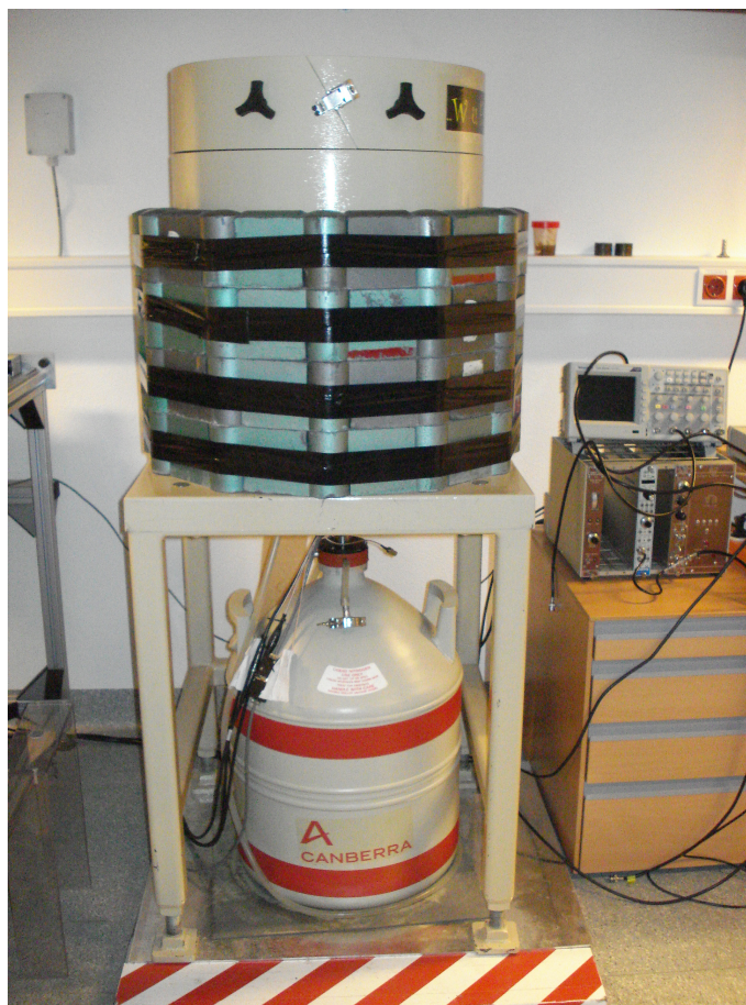
Figure 11.1: Gamma detector with additional shielding and liquid nitrogen cooling
