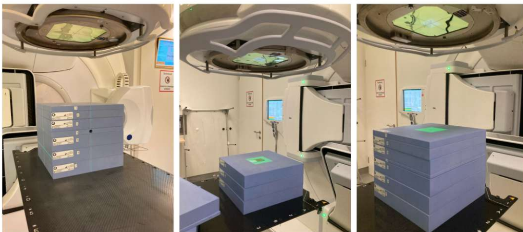
Fig. 2.10: Setup for the reference dosimetry and calibration measurement. First, the ionization chamber was inserted in the center for absorbed dose to water dosimetry (left), then the solid water was replaced to fit the radiochromic film at the same position (middle) before placing 10 cm thick slabs on top of the film for the measurement (right).
