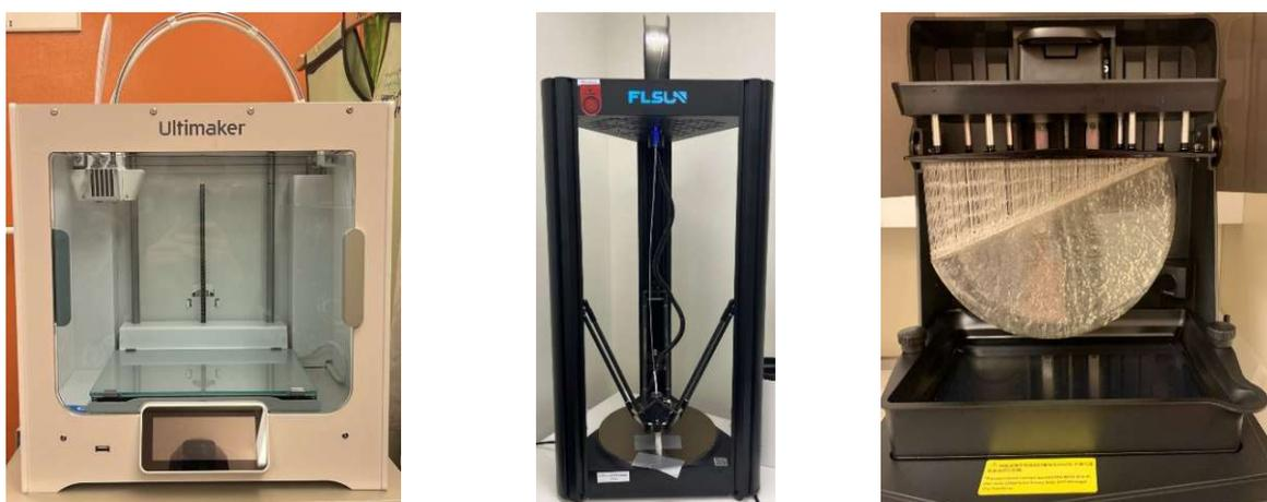
Figure 29: FDM Printers Ultimaker S3 (left), V400 by FLSUN (middle). SLA printer Saturn 4 Ultra by Elegoo with a completed print attached to the build plate (right).
