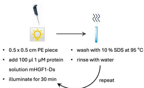
Figure 103| Design of the PE-degradation experiment with fusion protein mHGF1-DsFbFpM49I. a , ATR-FTIR analysis of desorption of mHGF1-DsFbFpM49I with 10 % ( \omega/v ) SDS at 95 °C. b , The PE sample was incubated for 0.5 h or 1 h with 1 \mu\text{M} protein solution (100 \mu\text{L} ) while illuminating with blue light (16.4 \text{mW}/\text{cm}^2 ). Subsequently, to remove the adsorbed protein, the PE piece was washed for 3 min in 10 % ( \omega/v ) SDS at 95 °C. It was rinsed with Milli-Q \text{H}_2\text{O} and dried with compressed air. All steps were repeated. In total, the sample was illuminated for approx. 148 h. c , The PE sample was incubated for 10 min with 25 \mu\text{M} protein solution (100 \mu\text{L} ) in the dark. Then, the solution was removed and dried with compressed air. It was illuminated for 20 min (16.4 \text{mW}/\text{cm}^2 ). Subsequently, to remove the adsorbed protein, the PE piece was washed for 3 min in 10 % ( \omega/v ) SDS at 95 °C. It was rinsed with Milli-Q \text{H}_2\text{O} and dried with compressed air. All steps were repeated. In total, the sample was illuminated for approx. 42 h.
