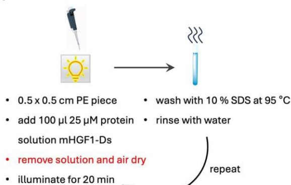
Figure 103| Design of the PE-degradation experiment with fusion protein mHGF1-DsFbFpM49I. a , ATR-FTIR analysis of desorption of mHGF1-DsFbFpM49I with 10 % ( \omega/v ) SDS at 95 °C. b , The PE sample was incubated for 0.5 h or 1 h with 1 \mu\text{M} protein solution (100 \mu\text{L} ) while illuminating with blue light (16.4 \text{mW}/\text{cm}^2 ). Subsequently, to remove the adsorbed protein, the PE piece was washed for 3 min in 10 % ( \omega/v ) SDS at 95 °C. It was rinsed with Milli-Q \text{H}_2\text{O} and dried with compressed air. All steps were repeated. In total, the sample was illuminated for approx. 148 h. c , The PE sample was incubated for 10 min with 25 \mu\text{M} protein solution (100 \mu\text{L} ) in the dark. Then, the solution was removed and dried with compressed air. It was illuminated for 20 min (16.4 \text{mW}/\text{cm}^2 ). Subsequently, to remove the adsorbed protein, the PE piece was washed for 3 min in 10 % ( \omega/v ) SDS at 95 °C. It was rinsed with Milli-Q \text{H}_2\text{O} and dried with compressed air. All steps were repeated. In total, the sample was illuminated for approx. 42 h.
