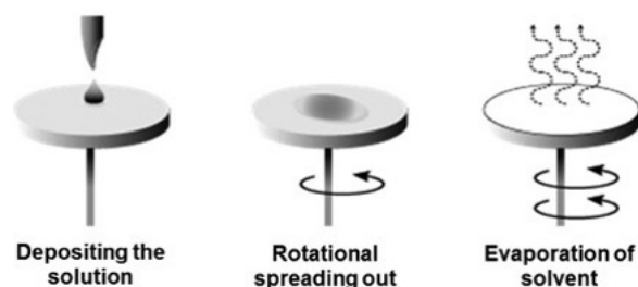
Figure 88| The principle of spin coating. The solution containing the dissolved polymer is deposited on the flat substrate. Then, rotation enables an even spreading out of the deposited solution while the solvent evaporates, and the polymer remains as a thin layer on the substrate. The figure was adapted from Amokrane et al. 200
