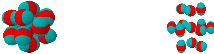
Figure 54: The unit cell of the investigated fcc-structure formed by spatial and orientational ordered IPCs is shown at a typical particle density (left) and at extremely large distances so that the orientation of the particles can be seen (right).
