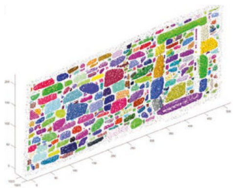
21 | Automated Segmentation of Individual Stones
