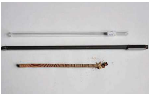
4 | Core Sample for determining the Age of the Wood
