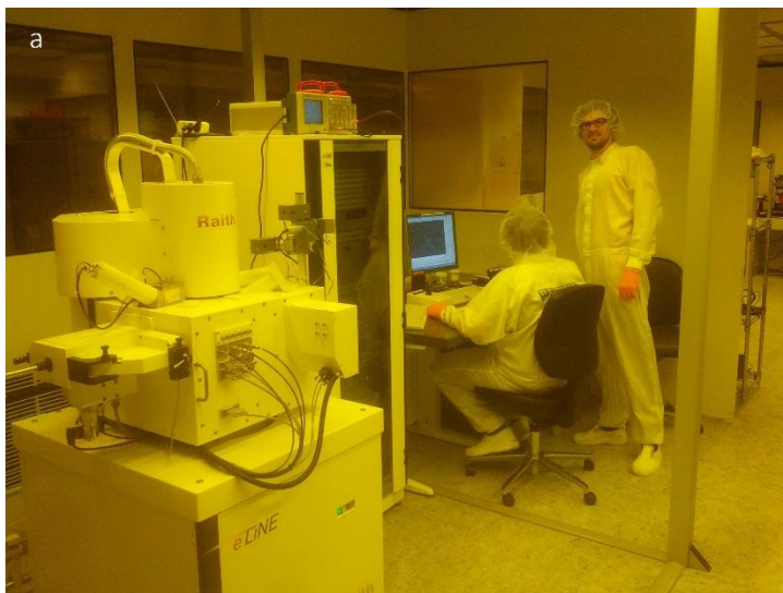
Figure 32: a: picture of the e-line writer in the cleanroom of the ZMNS at TU Vienna. b: Cross-section of structures written on PMMA with clearly overhanging edges. See [75].
