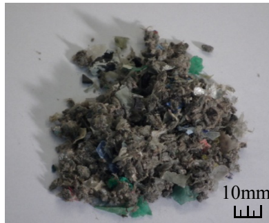
Figure 3.14: Processed waste plastics for injection into the blast furnace.
