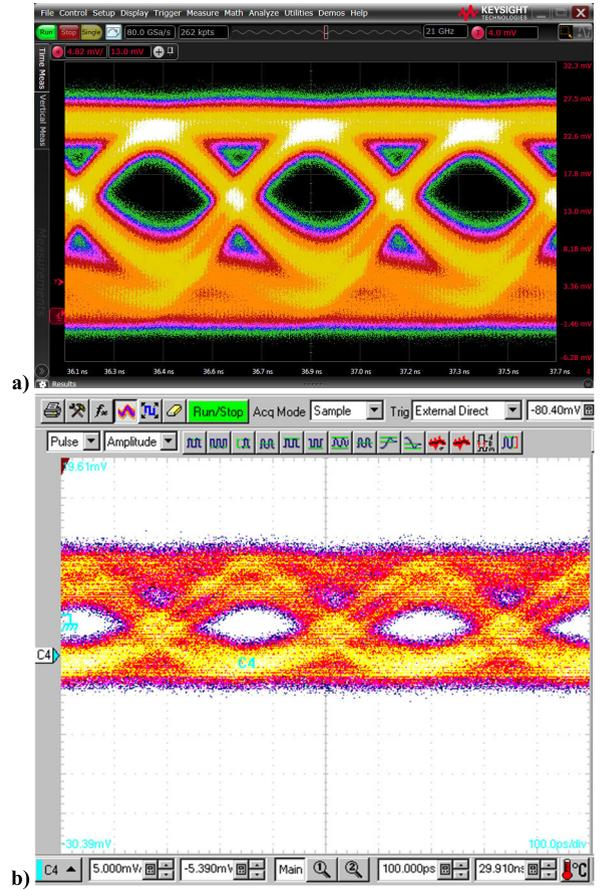
FIGURE 12. Measured eye diagrams at the TIA output for a) DR = 2 Gbps,  $I_{in} = 44 \mu A$  and PRBS31 (top), b) DR = 3 Gbps,  $I_{in} = 25 \mu A$  and PRBS7 (bottom).
