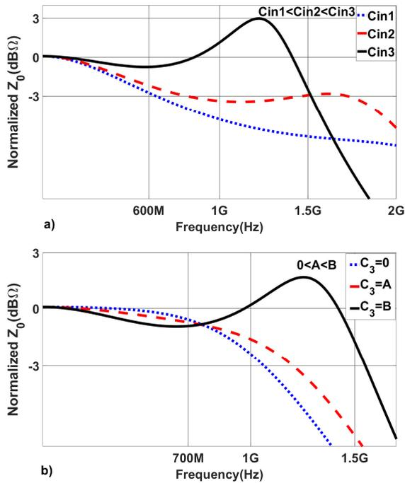
FIGURE 6. The effect of a)  $C_{in}$  and b)  $C_3$  values on the output impedance.
