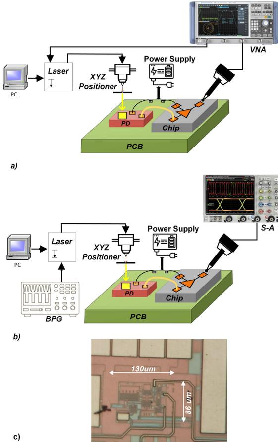
FIGURE 9. Measurement setup for a) frequency response, b) eye diagram, c) photomicrograph of fabricated chip.
