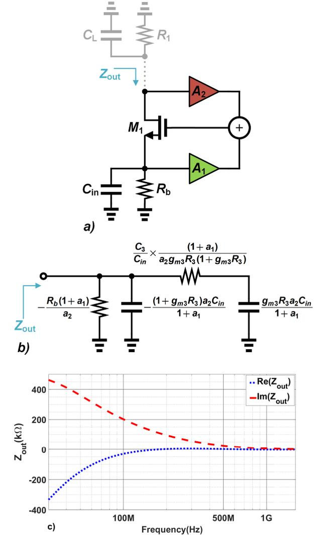
FIGURE 5. a), b) The equivalent model of the output impedance of the proposed topology, c) simulation results of the output impedance behavior.
