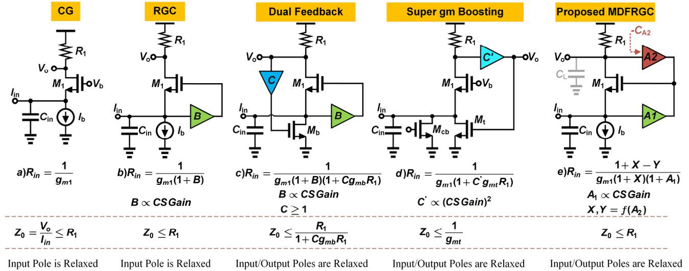
FIGURE 1. TIA topologies being employed to relax tradeoffs among the circuit parameters.
