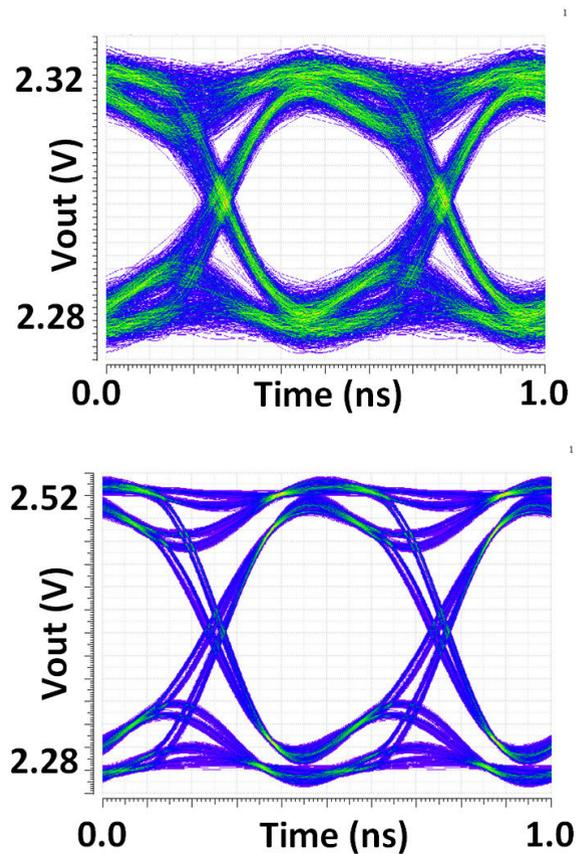
FIGURE 8. Simulated eye diagrams at the TIA output for DR = 2 Gbps and PRBS31 a)  $I_{in} = 11 \mu A$  (top), b)  $I_{in} = 70 \mu A$  (bottom).
