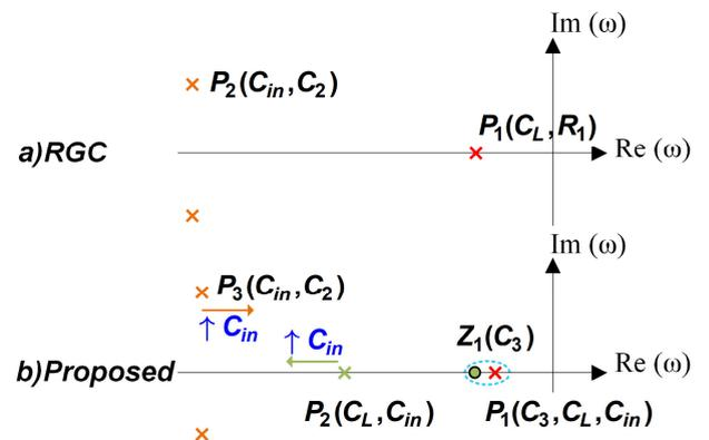
FIGURE 4. Pole-zero locations of (a) the RGC and (b) the proposed topology.
