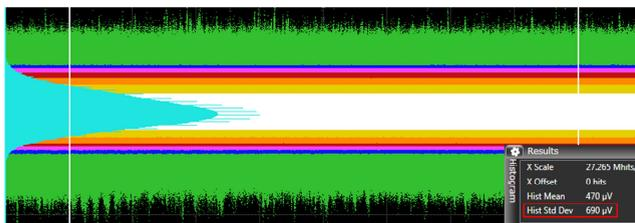
FIGURE 11. Output voltage histogram for dark conditions.
