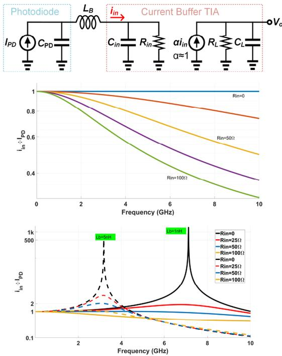
FIGURE 2. Simple PD and TIA connection model (top),  $I_{PD}$  and  $i_{in}$  currents transfer function for  $L_b = 0$  (middle) and for  $L_b$  variations (bottom).
