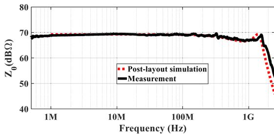
FIGURE 10. Frequency response and transimpedance gain of the proposed circuit with InGaAs PIN photodiode.
