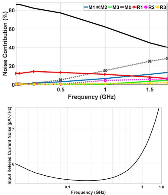
FIGURE 7. a) Noise contribution of circuit elements in the operating range (top), b) Input referred current noise (bottom).
