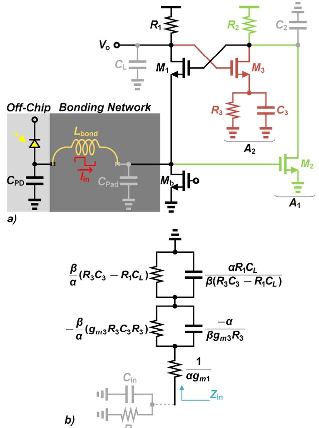
FIGURE 3. a) Circuit schematic of the proposed topology, b) model of the input impedance in the proposed topology.
