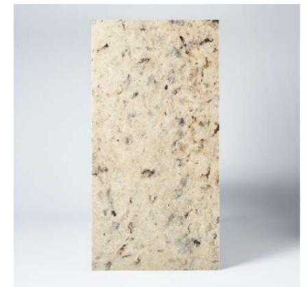
Abb. 17: Solid wool material sample, ©solidwool, 2023.
