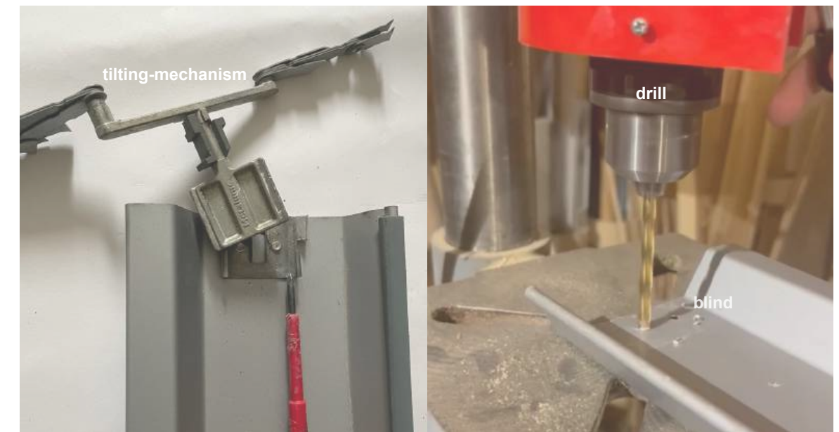
Fig.92 Taking off the tilting mechanism, unriveting the brackets
