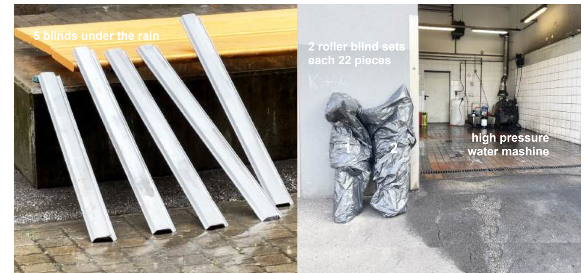
Fig.93 Cleaning with rain and afterwards with high-pressure water
