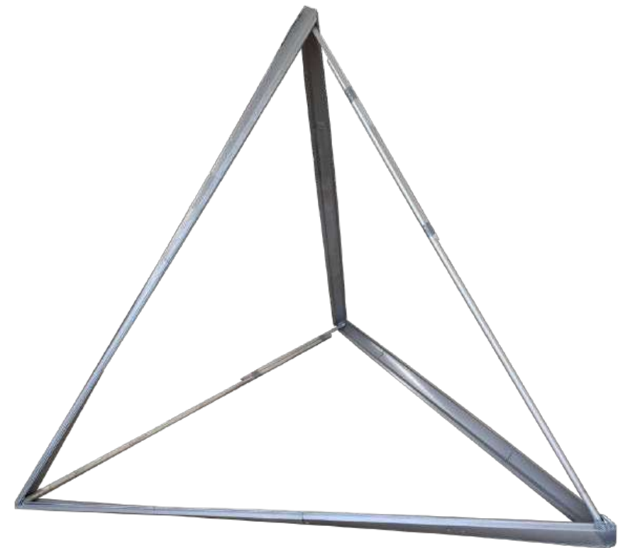
Fig.105 A finished frame with supporting rods forming a tetrahedron.
