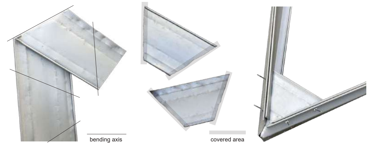
Fig.123 Process of building the angles: bending the flattened blind, plates, riveting of the angles
