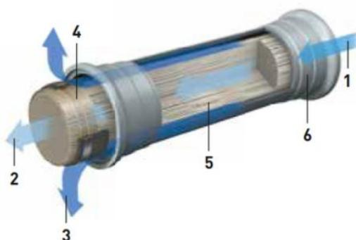
Schematic representation of a hollow-fiber module
