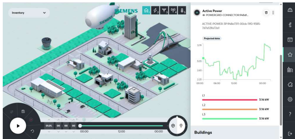
Figure 2.1: The web-based interface of the BIFROST simulation environment with an exemplary settlement, showing different buildings and landscape elements, as well as the plot illustration of variables within the GUI
