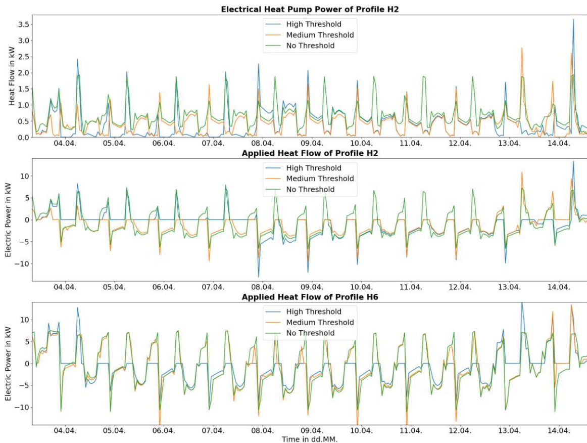
Figure 5.3: HPs electrical power for three different switching thresholds of HP's operation mode for profile H2, as well as the applied heating flow for profile H2 and H6 from April 4 th to April 14 th
