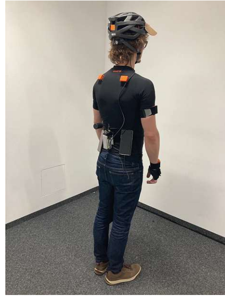
Figure 2.8: Equipped Participant from the back with eye-tracker phone and GNSS phone attached next to the GNSS antenna.
