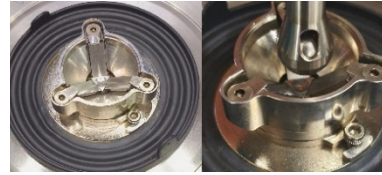
Figure 2. Three plate geometry sample holders.
