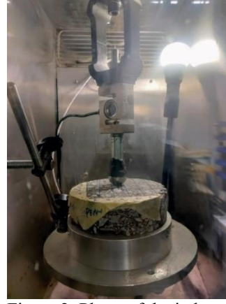
Figure 2. Photo of the indentation test setup.
