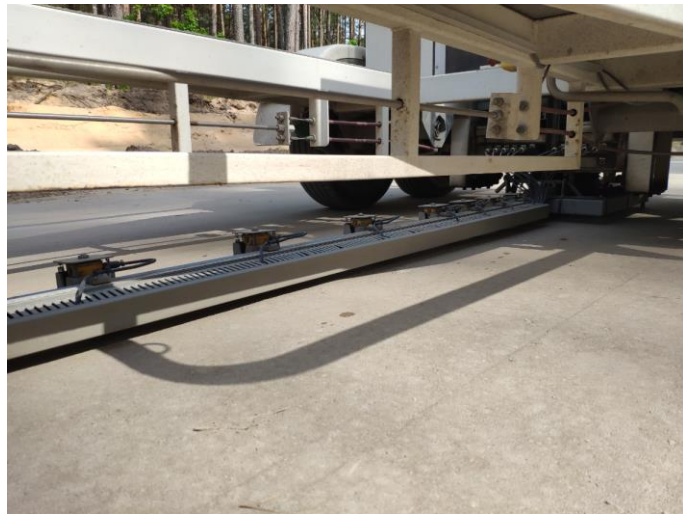
Figure 2. Pavement bearing capacity measurements with FWD.
