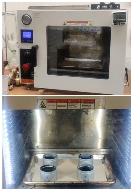
Figure 2. Vacuum oven used for recovery of binder from the binder-solvent solution.
