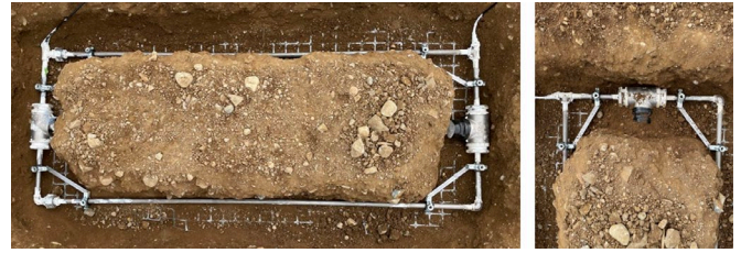
Figure 5: Bender Element (BE) field sensor installed in-situ.
