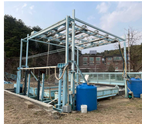
Figure 3. Rainfall Simulator (a) Experiment conditions (b) Actual Rainfall Simulator
