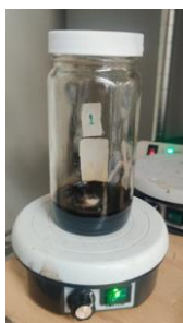
Figure 1. Binder pellet dissolved in a solvent in a glass bottle stirred on a magnetic stirrer.
