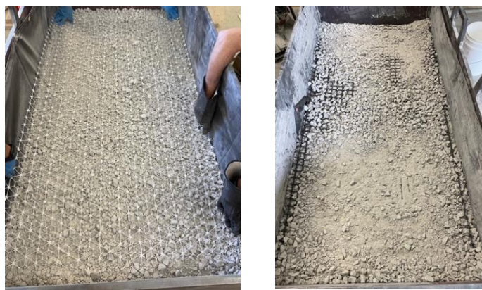
Figure 3. Geosynthetic placement in large-scale testbed.
