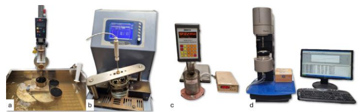
Figure 4. a) Penetration test b) Softening point test c) Viscometer Brookfield d) Dynamic Shear Rheometer (DSR)
