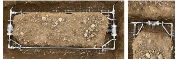
Figure 5: Bender Element (BE) field sensor installed in-situ.
