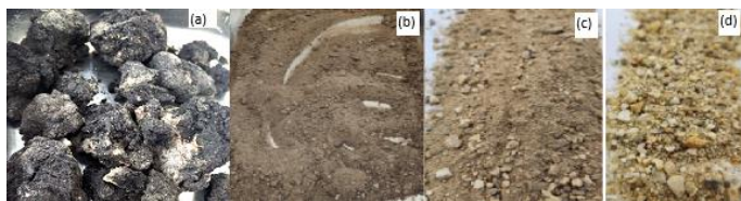
Figure 1. Materials (a) contaminated oil sand – natural state (b) CS (c) limestone dust (d) sharp sand.
