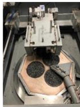
Figure 1. Arrangement of RSAT plates and test setup.
