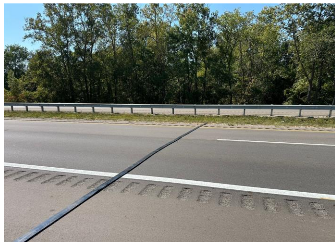
Figure 2. Strip laid across the road width at US 127, Mason, adjacent to a WIM system.
