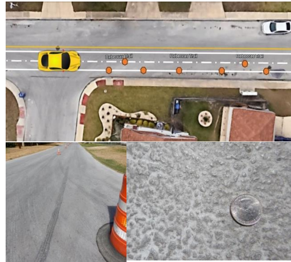
Figure 2. Typical measurement locations relative to traffic direction and photo cool pavement treatment (Product C).
