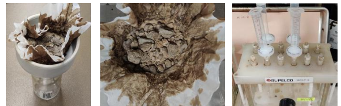
Figure 4. Trial with coffee filter as the first stage in the two-step filtration and vacuum manifold with syringe filters
