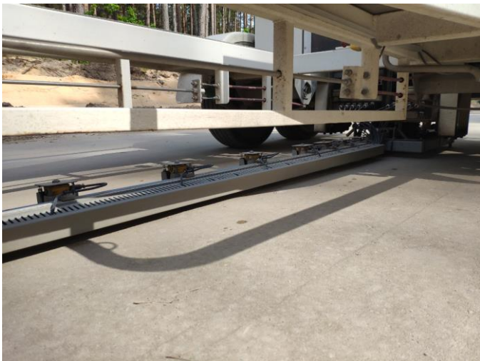
Figure 2. Pavement bearing capacity measurements with FWD.
