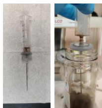
Figure 5. Manual method of drawing supernatant through a syringe filter from the undisturbed solution (without vacuum assistance and stirring)
