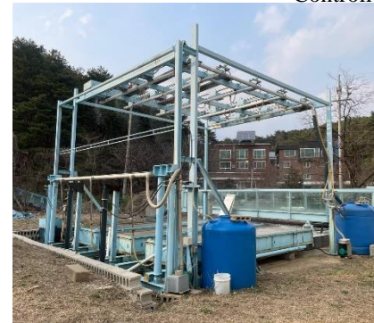
Figure 4. Measurement of WFT using Water Film Gauge
