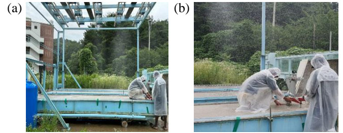
Figure 7. (a) Distant view of British Pendulum Number measurement in wet conditions, (b) Close-up view of British Pendulum Number measurement in wet conditions.
