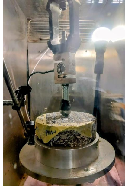
Figure 2. Photo of the indentation test setup.
