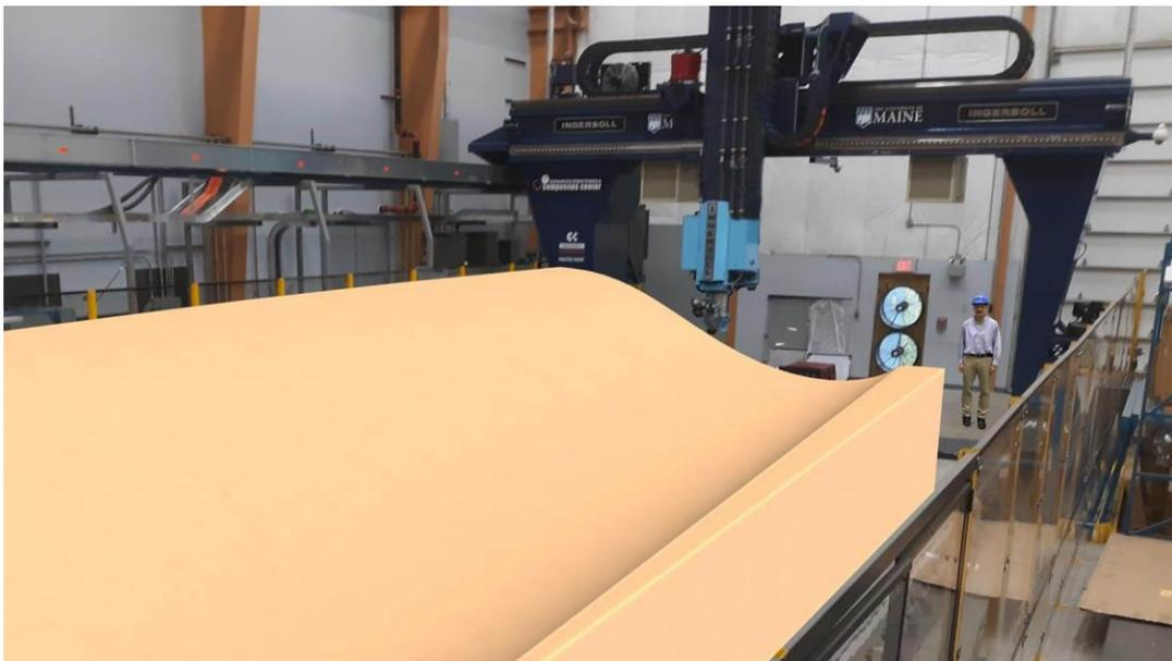
Figure 15 A 3D printed wind blade mould. Image courtesy of UMaine
