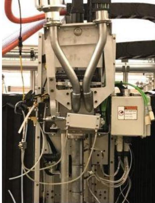
Figure 2 dual-hopper system on the MDF's BAAM-B
