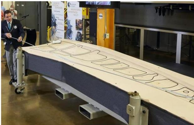
Figure 12 The 3D printed trim tool co-developed by Oak Ridge National
