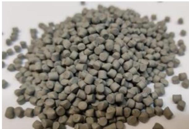
Figure 6 MIM granulates used for 3D printing
