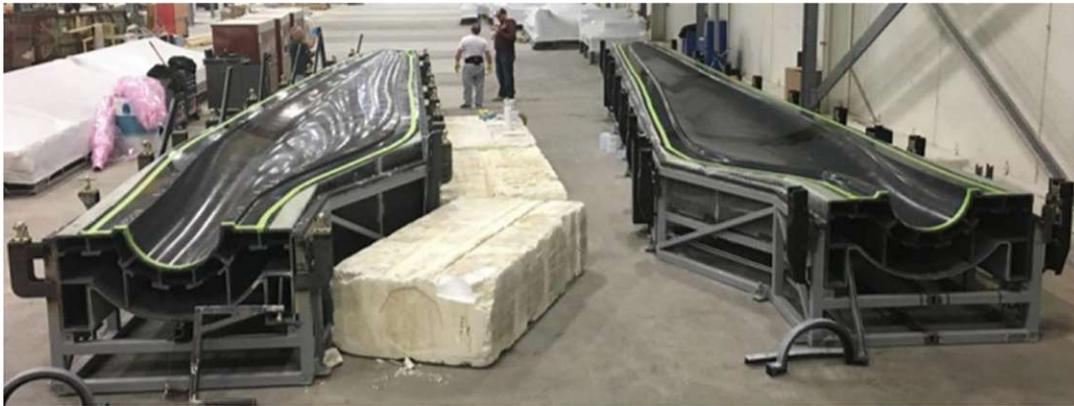
Figure 16 3D printed wind turbine mould by ORNL
