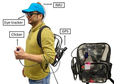
(b) A participant equipped with an eye-tracker, an IMU attached to the cap, a GPS receiver on the backpack, and a handheld clicker connected to an LED light attached to the backpack. The participant has provided written permission for the use of his photo in publications.
