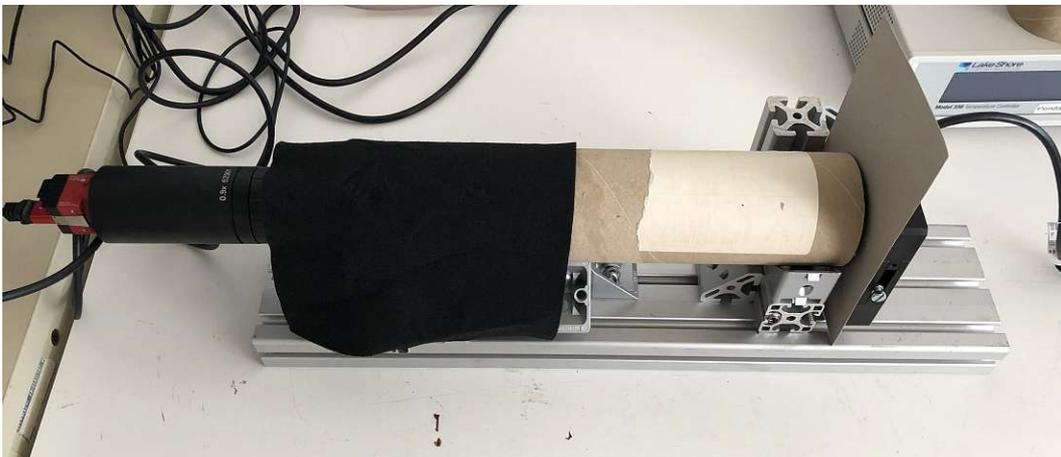
**Figure 4.6.47:** A picture of the optical calibration setup with the covers on. The tube has a small hole in the bottom to allow the calibration ball to go in. on the right there is one of the various shutter sheets we produced in position. they were placed there to test the influence of the light sources size on the fitting quality.
