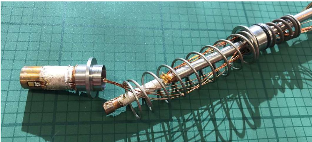
**Figure 4.3.28:** The inside of the cold finger put together. For final assembly of the cold finger the tip heater will be put through the counter heater so that the long spring is compressed by the counter heater adaptor that in this picture is already connected to the counter heater by tight fit on the adaptor. This spring is for spring loading the counter heater to improve thermal contact there to. The wires are put through the holes in the spine according to [4.3.27](#).
