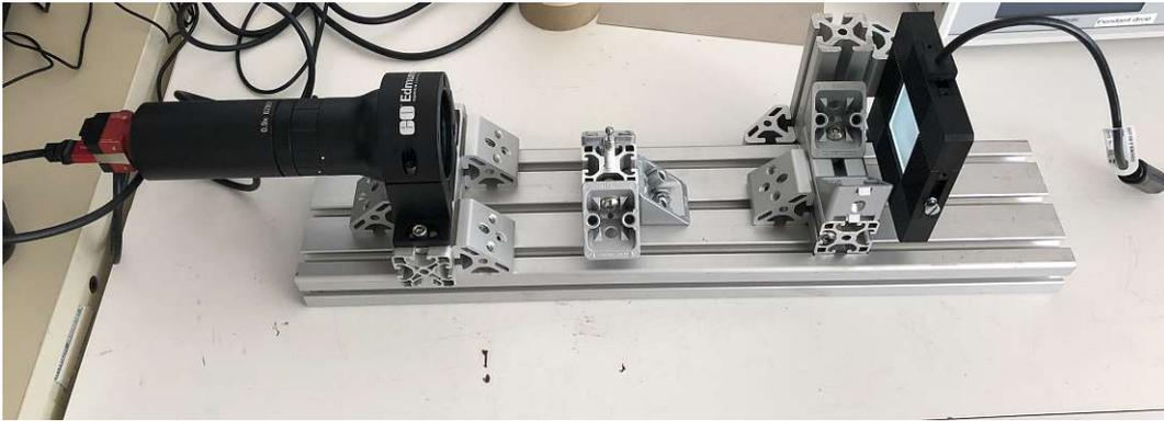
**Figure 4.6.46:** A picture of the optical calibration setup without the cover. On the left there is the lens with the camera attached to it and on the right the back illumination. In the middle on a small post there is the calibration ball.
