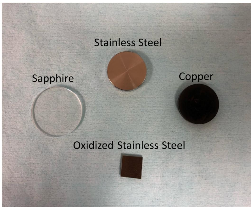
**Figure 7.3.58:** This figure shows the 4 material samples after the experiments.
