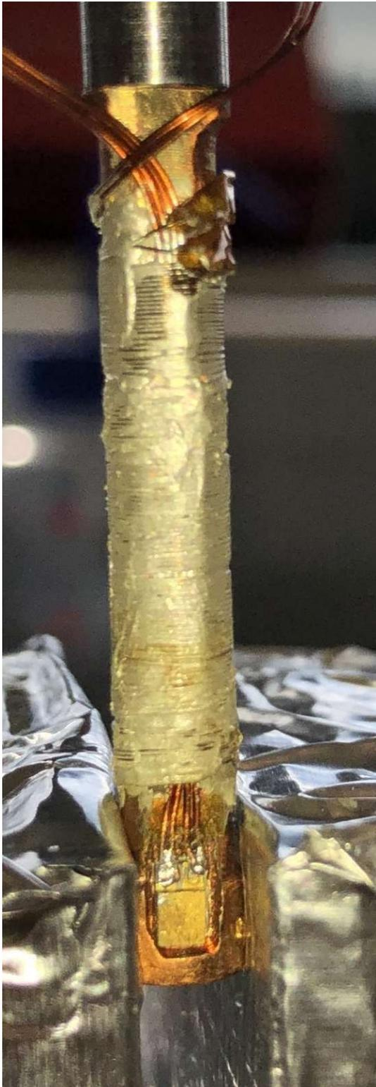
(a) The finished tip heater. Here different to the counter heater the connection between the manganin and the copper wire was insulated by capton tube. The space around the tip heater is more restrictive than around the counter heater and the shrink tube would not fit. Other than that it was done in the same way. 47
