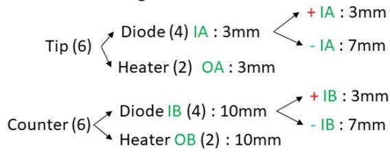
The wires are bundled up and marked with shrinktube pieces of different length. The organigram to the left explains which length corresponds to which wirebundle. The number in the brackets corresponds to the amount of wires going through the shrinktube.
