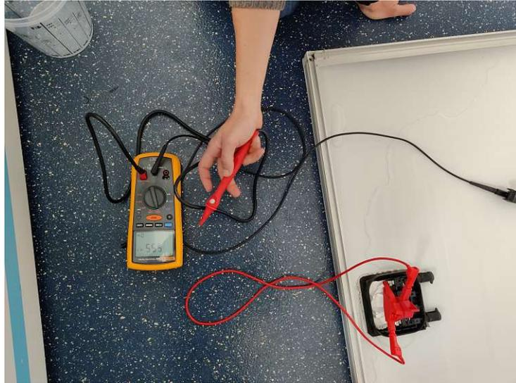
Figure 4.18: Test-setup for wet leakage test
