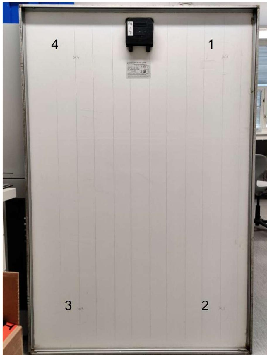
Figure 4.1: Overview of the Kioto 235Wp PV module with cracked BS. The numbers refer to the sample areas where the four repair materials were applied
