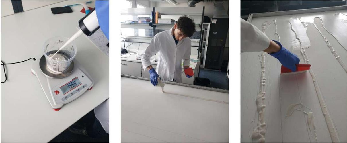
Figure 4.13: First steps of the silicone coating process
