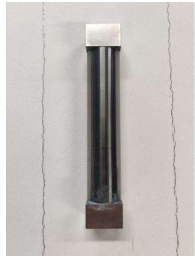
(c) Coating knife used for applying coating with specific layer thickness
