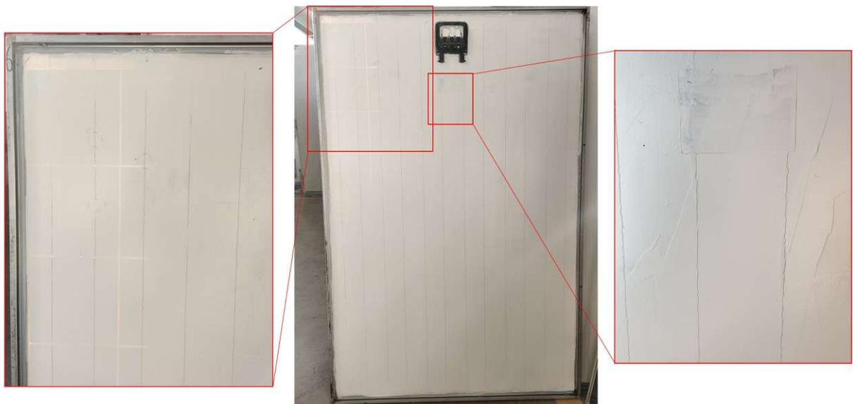
Figure 4.34: The optimized PU coating on Module M6 after 25 TC with the modified application and test parameters
