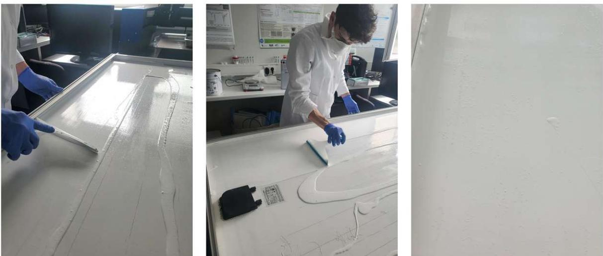
Figure 4.16: Application of the cover coating in the Remisol coating process
