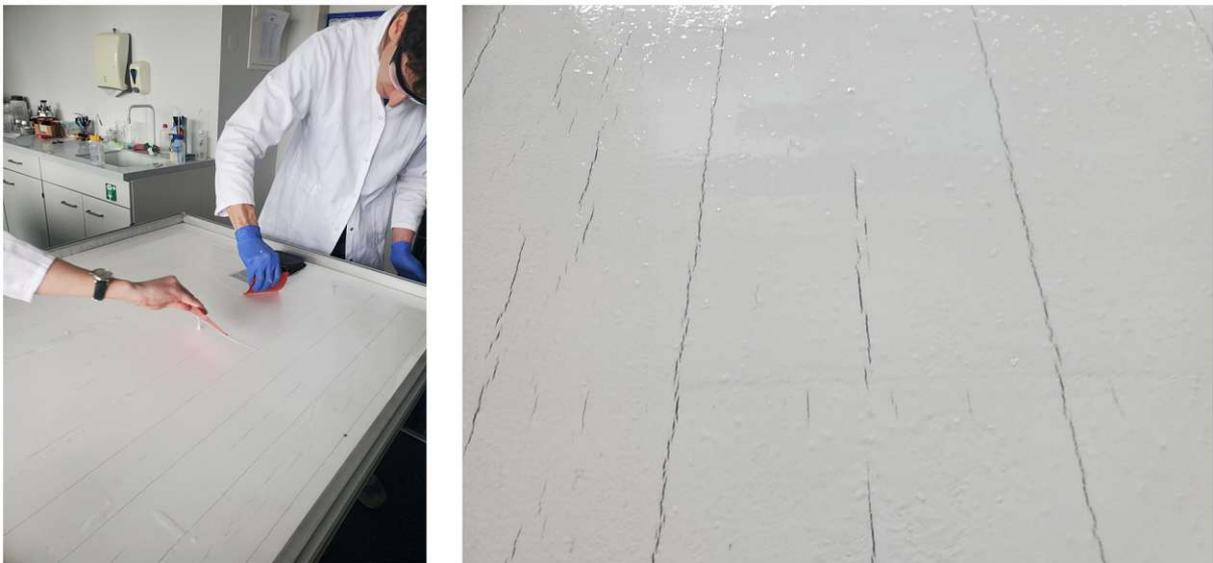
Figure 4.15: Application of the crack filler in the Remisol coating process
