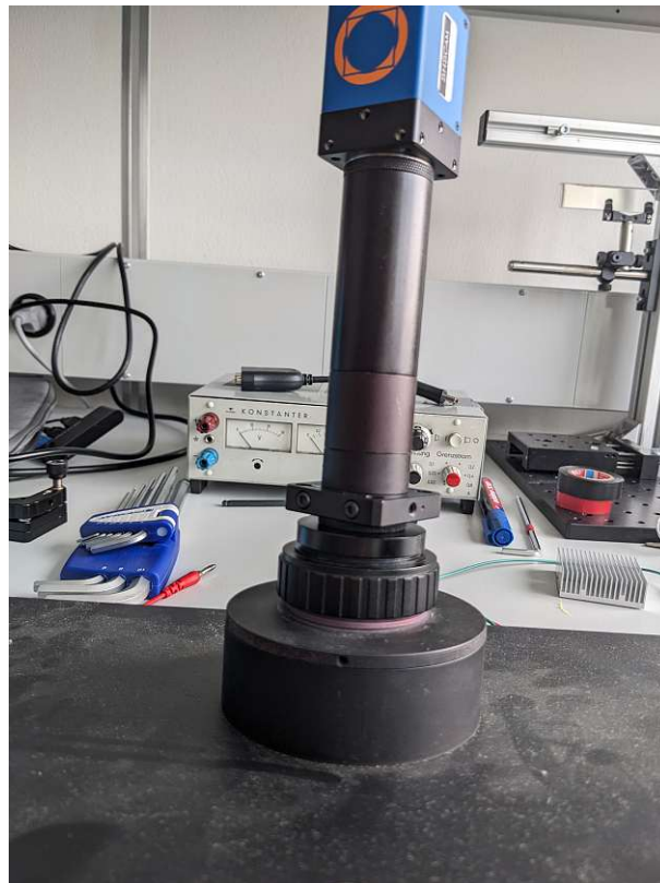
Figure 5.10: Connection between the WFS and the backplate of the telescope.
