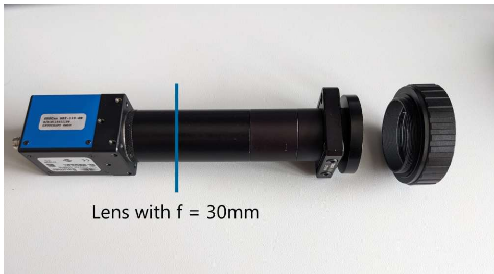
Figure 4.8: SHWFS and adapter tube with collimating lens.
