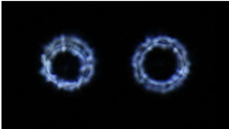
Figure 4.6: Star test, where the SM is misaligned (left) and after adjustment (right) [51].
