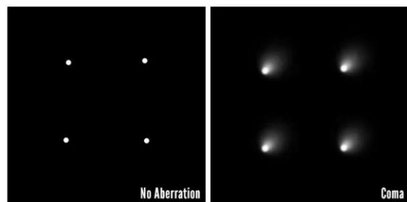
Figure 3.5: Light path in case of coma [16]. Figure 3.6: Picture visualising the effect of coma [46].
