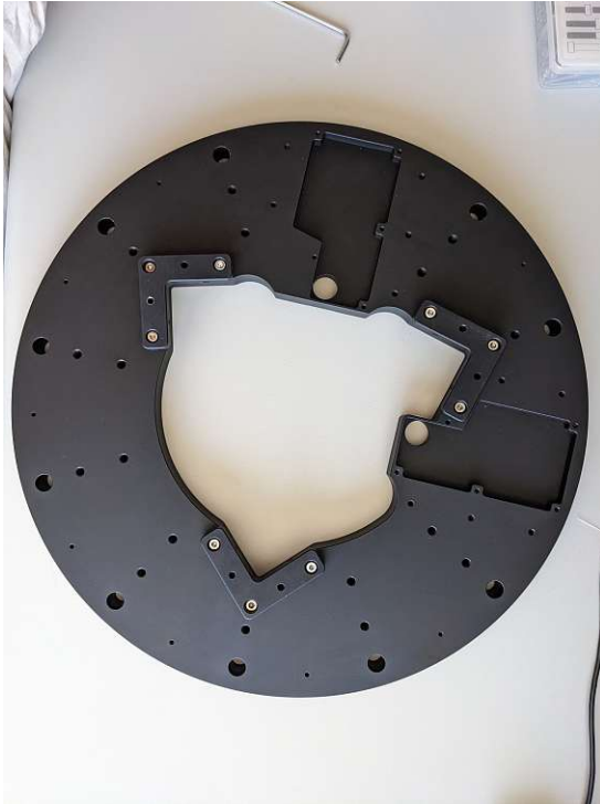
Figure 5.3: Manufactured PM ring adapter.
