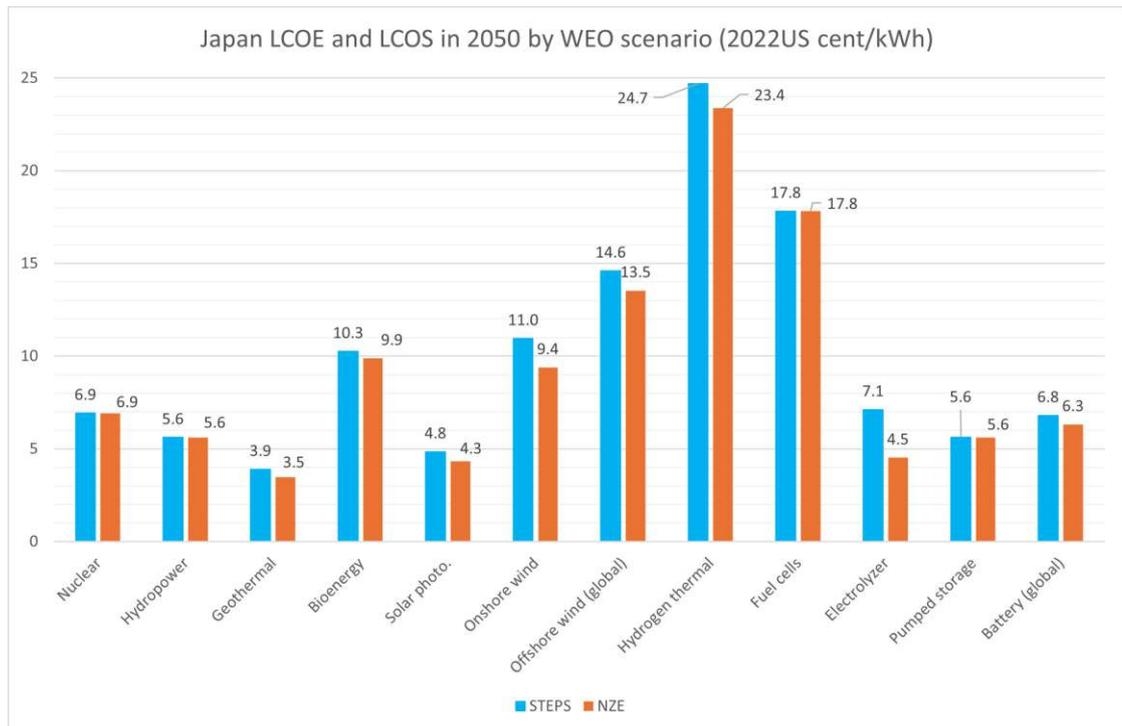
Figure 6.1: Levelized costs of electricity and storage in Japan in 2050 by WEO scenario
