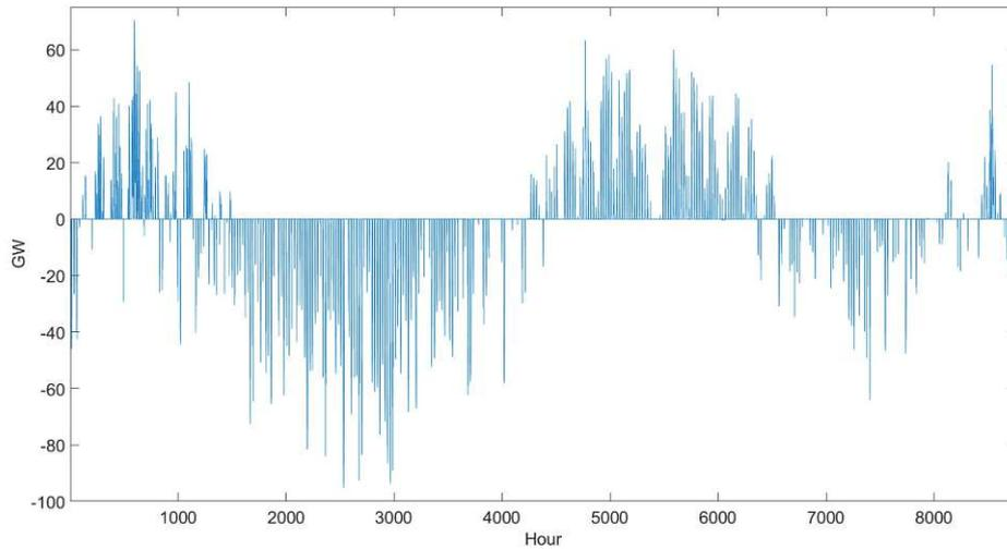
Figure 5.9: The *netval* vector represents the discrepancy between electricity demand and supply for each hour of the year. This Figure illustrates the maximum demand in 2050 minus the supply under a 60% renewable energy share target, as outlined to Japan's plan, referred to as Scenario 0 in this thesis (see Table 5.3).
