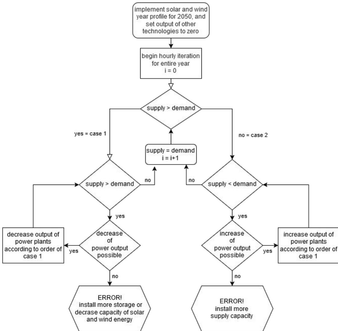
Figure 5.8: Conceptual flowchart of the algorithm
