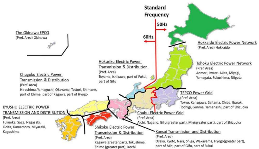
Figure 2.1: Japan's electricity grid with two different frequency zones and ten smaller grids, each operated by one of the electric companies of Japan. (Source: OCCTO, 2022a)
