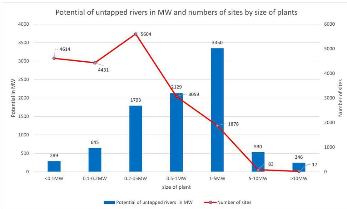
Figure 3.2: Hydropower potential according to the Ministry of Environment Survey in 2011 (Source: MOE, 2012)
