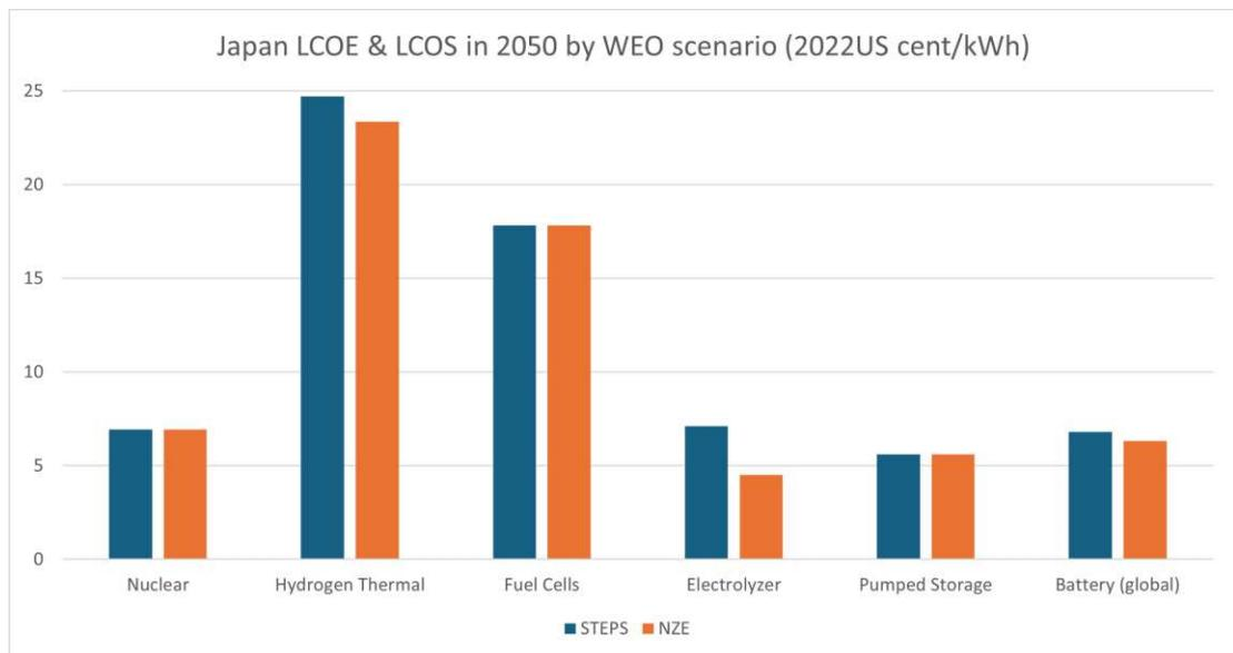
Figure 4.4: Levelized costs of electricity and storage in Japan in 2050 by WEO scenario
