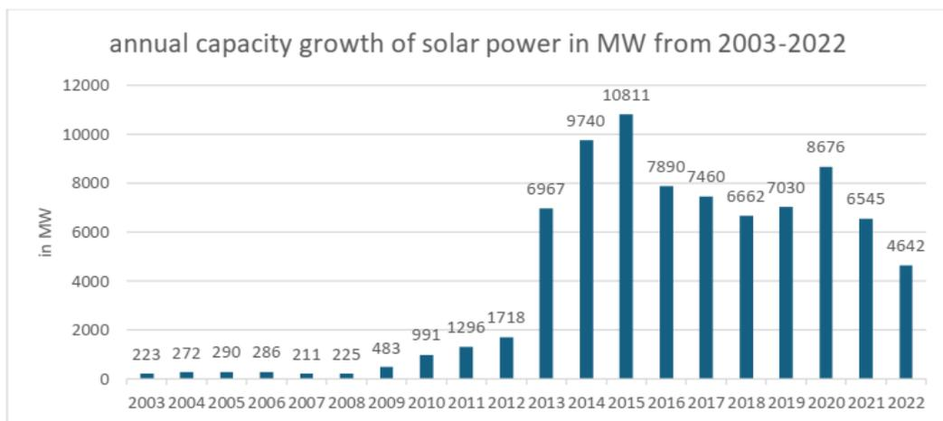
Figure 3.6: The effects on the installation rate of solar photovoltaic energy after the new FiT was introduced in 2012 (based on: IRENA, 2024b)
