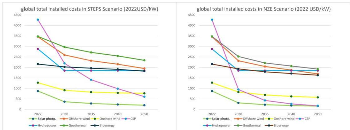
Figure 4.1: Global total installed costs in STEPS and NZE Scenario in (2022 USD / kW)
