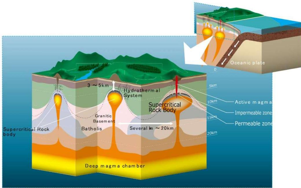
Figure 3.4: Conceptual model of the super critical geothermal system in northeast Japan (Source: Asanuma et al., 2021) - Supercritical Rocky Bodies are supposed to be in shallower depths in volcanic areas making it easier for access.
