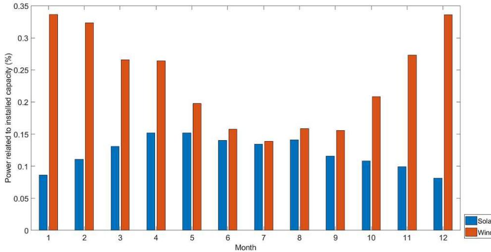
Figure 5.6: Monthly mean profiles of solar and wind power related to installed capacity between 2017-2023
