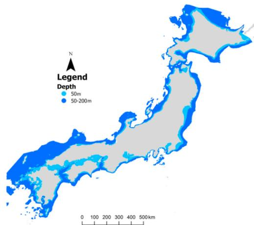
Figure 3.9: Offshore wind energy potential around Japan by zones of water depth:  $\leq 50$  m in light blue; 50 - 200 m in sky blue (Source: Bardenhagen and Nakata, 2020)
