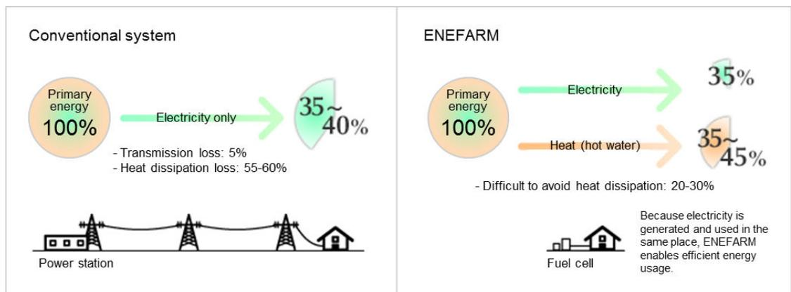
Figure 3.12: Concept of the "ENE-Farm" home fuel cell: Enhancing total energy efficiency by eliminating heat losses (Source: ITOCHU ENEX Co.LTD., 2024)
