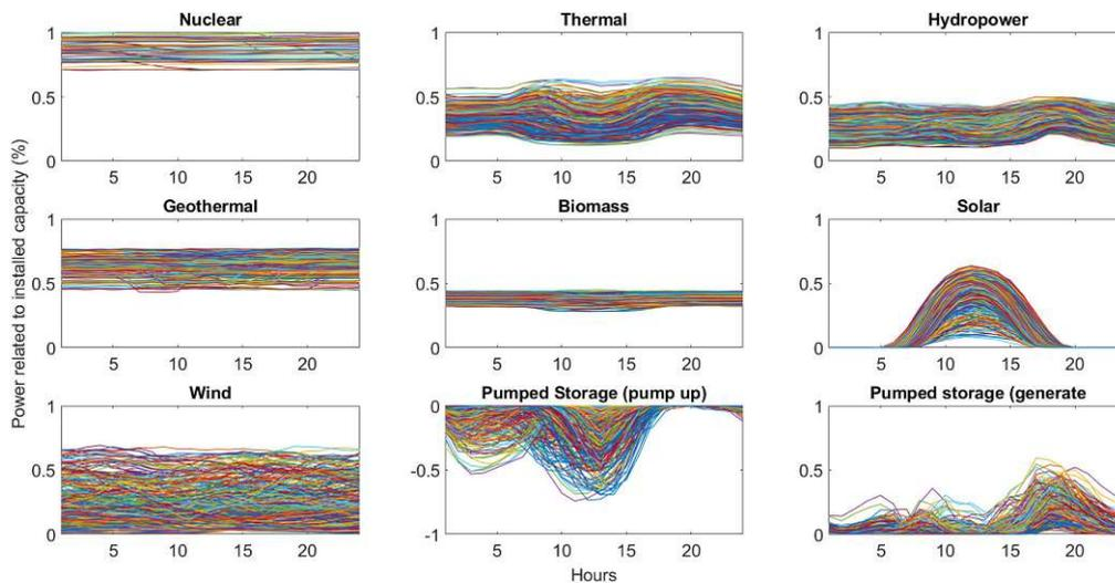
Figure 5.4: Daily profiles of electricity supply related to installed capacity in 2023 by technology
