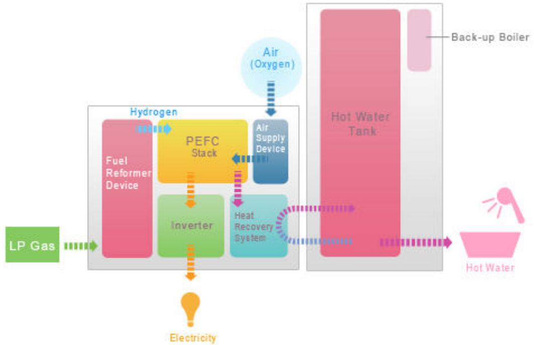
Figure 3.11: The structure of the "ENE-Farm" home fuel cell (Source: JAPAN LP Gas Association, 2024)
