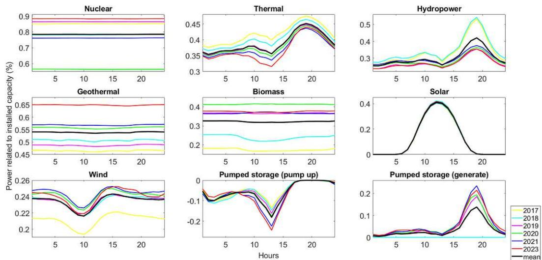
Figure 5.5: Daily average profiles of electricity supply from different technologies, calculated per year, during the period 2017–2023.
