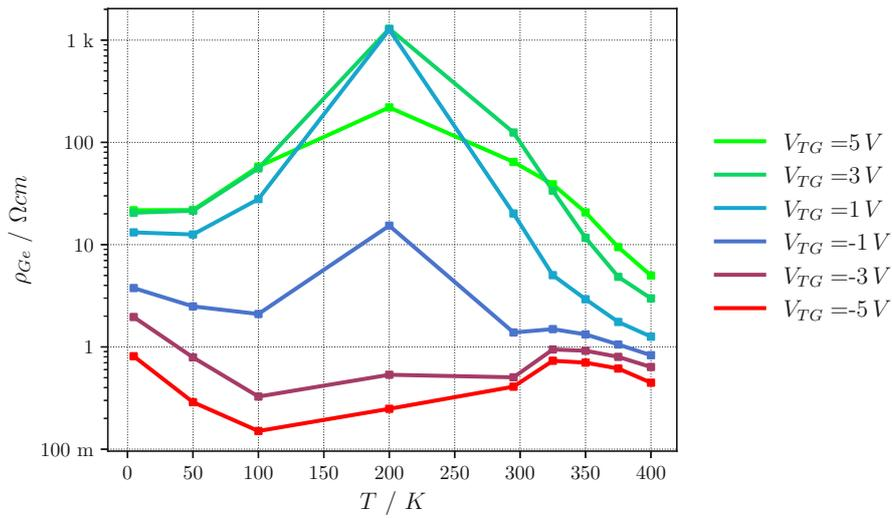
**Figure 4.16:** Device resistivity of device 10\_12 ( $l_{Ge} = 0.15 \mu m$ ) as a function of temperature and top-gate voltage calculated on the linear portion of the previously recorded I-V characteristics. The gate voltage ranges from  $-5 V$  to  $+5 V$ , with a voltage spacing of  $2 V$ , while the temperature varies from  $4.8 K$  to  $400 K$ .  $\rho_{Ge}$  is presented in a logarithmic format.
