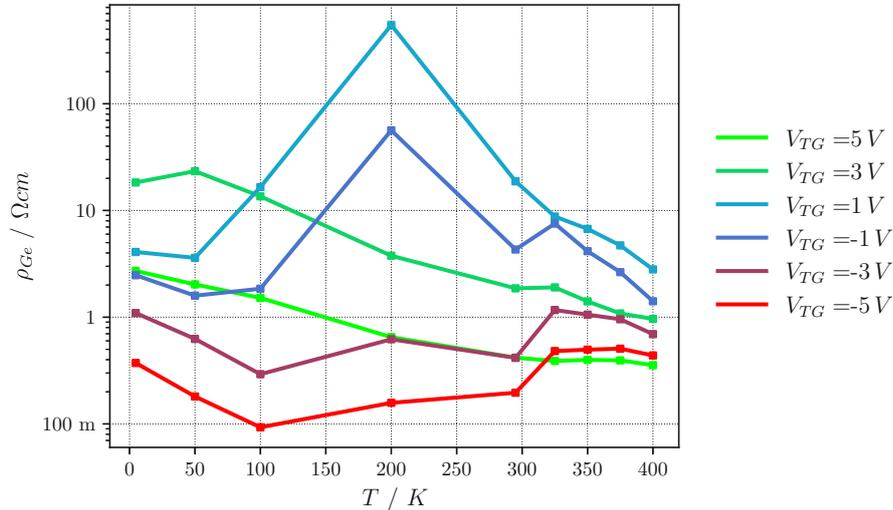
**Figure 4.6:** Device resistivity of device 03\_00 ( $l_{Ge} = 102\ \mu\text{m}$ ) as a function of temperature and top-gate voltage calculated on the linear portion of the previously recorded I-V characteristics. The gate voltage ranges from  $-5\text{ V}$  to  $+5\text{ V}$ , with a voltage spacing of  $2\text{ V}$ , while the temperature varies from  $4.8\text{ K}$  to  $400\text{ K}$ .  $\rho_{Ge}$  is presented in a logarithmic format.
