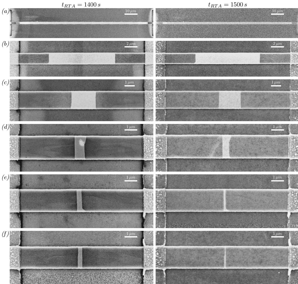
**Figure 4.1:** SEM images of the Ge nanosheet after 1400 s and 1540 s of RTA. The devices are identified as (a) 03\_00, (b) 05\_13, (c) 11\_03, (d) 11\_08, (e) 10\_12, and (f) 08\_03. Their dimensions, such as the gap between the Al pads,  $l_{Ge}$ , and the width of the sheet structures, can be found in Table 4.1.
