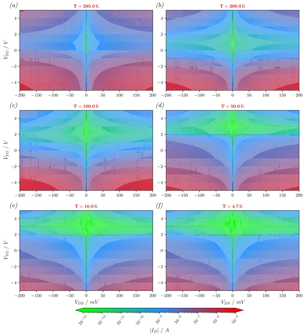
**Figure A.3:** The  $I$ - $V$  characteristics of device 05\_13 ( $l_{Ge} = 10 \mu\text{m}$ ) are presented as a function of temperature, bias, and top-gate voltage, shown as  $|I_D(V_{DS}, V_{TG})|$  in a logarithmically scaled colormap. The temperature dependence can be understood by interpreting each subplot from top to bottom as corresponding to decreasing temperature.
