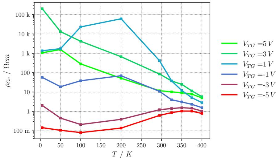
**Figure 4.11:** Device resistivity of device 11\_03 ( $l_{Ge} = 2\ \mu\text{m}$ ) as a function of temperature and top-gate voltage calculated on the linear portion of the previously recorded I-V characteristics. The gate voltage ranges from  $-5\ \text{V}$  to  $+5\ \text{V}$ , with a voltage spacing of  $2\ \text{V}$ , while the temperature varies from  $4.8\ \text{K}$  to  $400\ \text{K}$ .  $\rho_{Ge}$  is presented in a logarithmic format.
