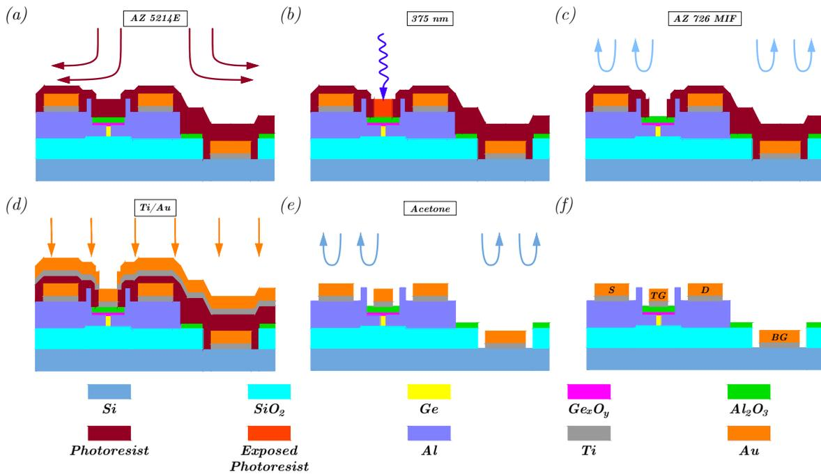
**Figure 3.7:** Illustration of the top-gate deposition process: (a) Spin-coating of AZ 5214E photoresist, (b) positive lithography process, (c) developing of photoresist, (d) physical vapor deposition of 10 nm Ti and 100 nm Au via electron-beam evaporation, (e) removal of excess Ti and Au material through a lift-off process, (f) completion of the sample fabrication process. The device's electrical contacts are labeled as drain (D), source (S), top gate (TG), and back gate (BG).
