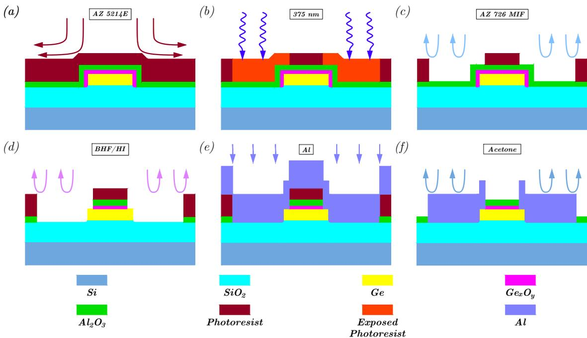
**Figure 3.4:** Schematic sequence of the fabrication of the Al pads, to contact the Ge sheets: (a) Spin-coating of AZ 5214E photoresist. (b) Positive lithography process to form the openings for the deposition of Al. (c) Development of the illuminated resist areas. (d) Wet-chemical etching of the  $Al_2O_3$  and native  $Ge_xO_y$ . (e) Al sputtering onto the sample. (f) Lift-off process in acetone to eliminate the photoresist and the excessive Al.
