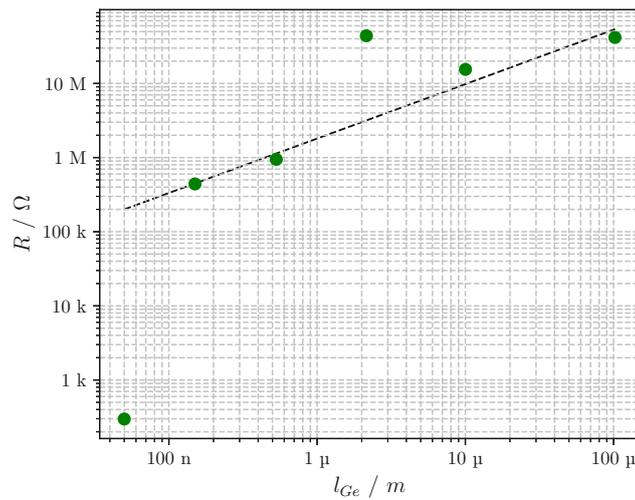
**Figure 4.20:** The resistance is represented as a function of the length of the Ge segment, displayed in a double logarithmic format.
