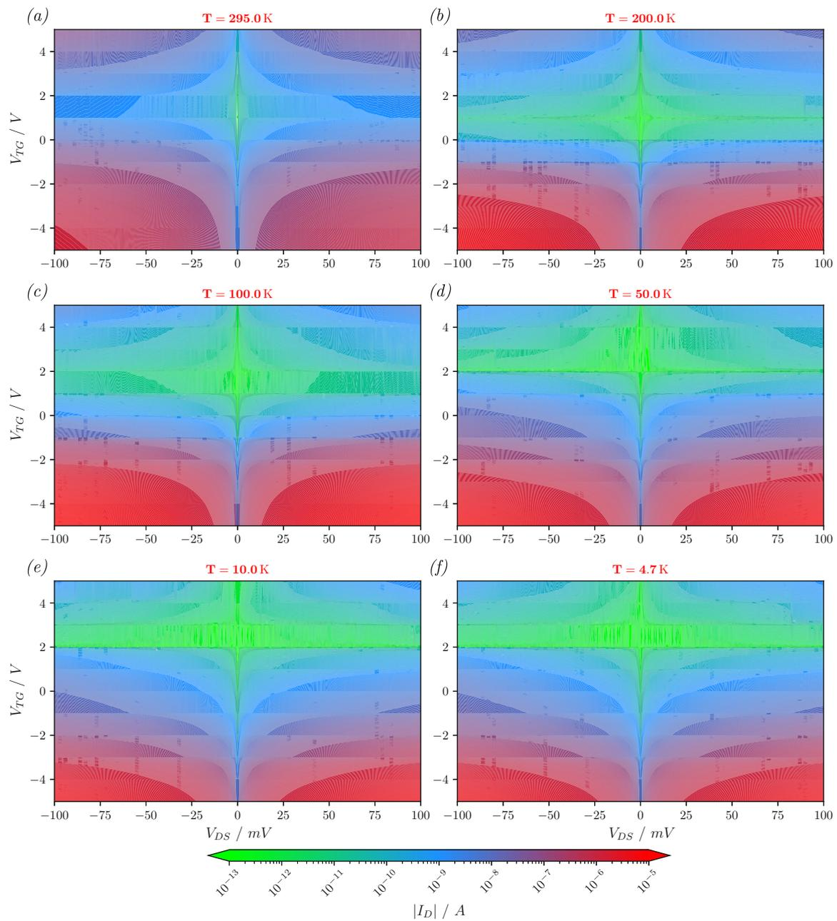
**Figure 4.10:** The  $I$ - $V$  characteristics of device 11\_03 ( $l_{Ge} = 2 \mu\text{m}$ ) are presented as a function of temperature, bias, and top-gate voltage, shown as  $|I_D(V_{DS}, V_{TG})|$  in a logarithmically scaled colormap. The temperature dependence can be understood by interpreting each subplot from top to bottom as corresponding to decreasing temperature. Image based on [128].
