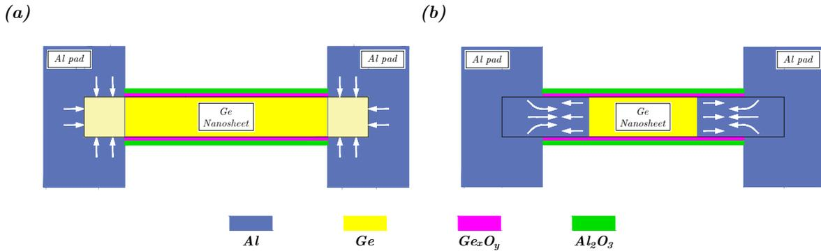
**Figure 2.6:** The outlined illustration depicts the solid-state diffusion process in Al-Ge-Al nanosheet heterostructures. In subfigure (a), the initial state is shown, where Ge starts to diffuse into the Al pads. (b) illustrates the formation of two Kirkendall planes within the nanosheet, oriented perpendicular to the diffusion direction. As diffusion progresses, both atomically sharp Al-Ge interfaces gradually shift toward the center of the nanosheet. Image adapted from [48, 107].
