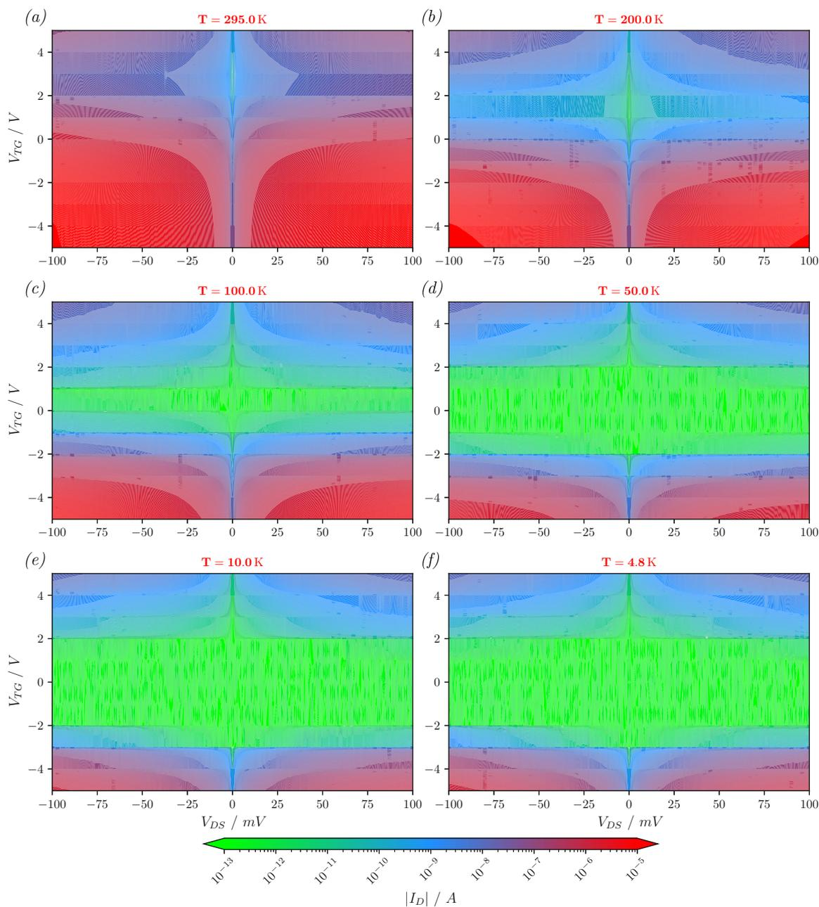
**Figure A.4:** The I-V characteristics of device 11\_08 ( $l_{Ge} = 0.5 \mu\text{m}$ ) are presented as a function of temperature, bias, and top-gate voltage, shown as  $|I_D(V_{DS}, V_{TG})|$  in a logarithmically scaled colormap. The temperature dependence can be understood by interpreting each subplot from top to bottom as corresponding to decreasing temperature.
