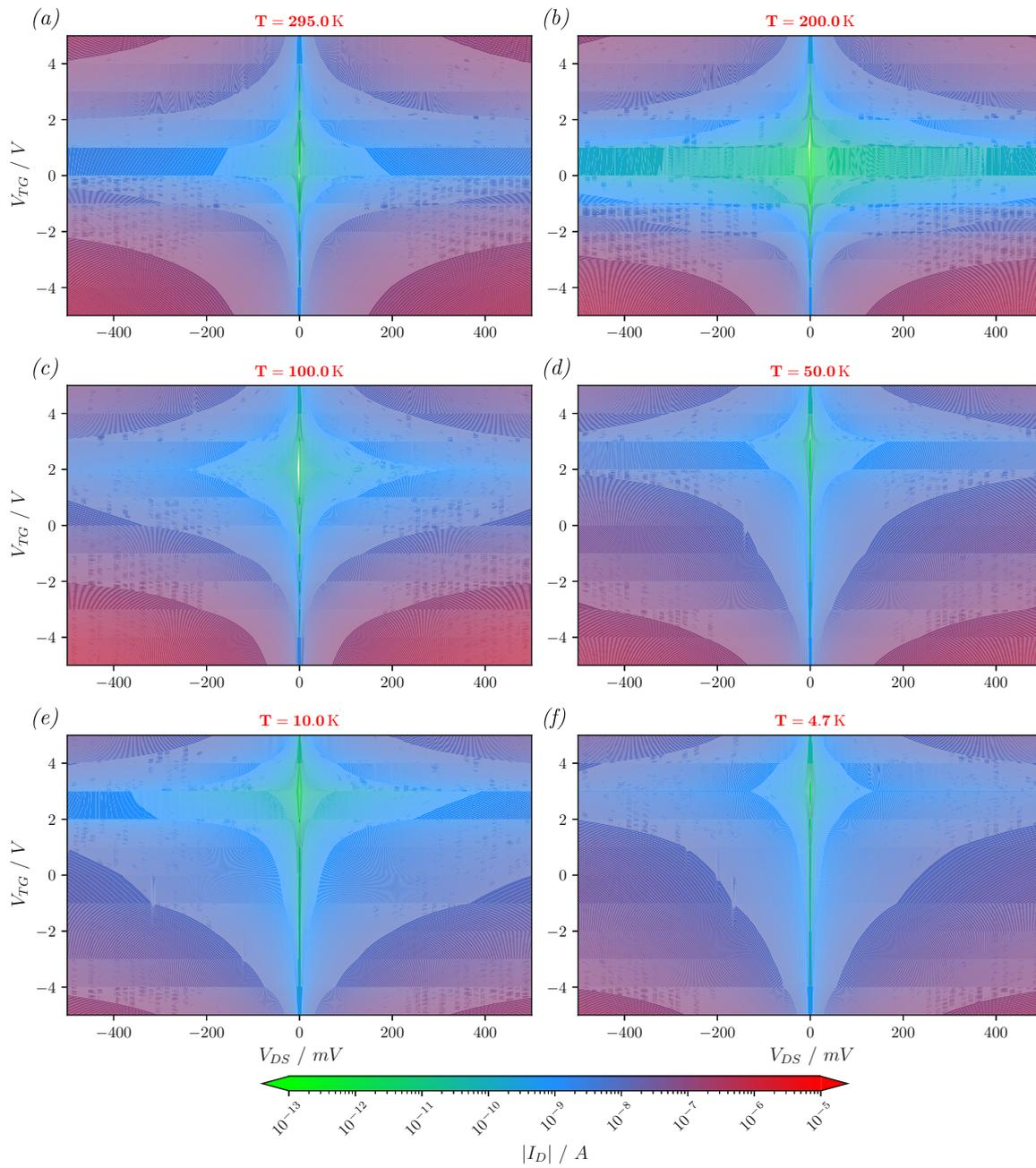
**Figure 4.5:** The  $I$ - $V$  characteristics of device 03\_00 ( $l_{Ge} = 102 \mu\text{m}$ ) are presented as a function of temperature, bias, and top-gate voltage, shown as  $|I_D(V_{DS}, V_{TG})|$  in a logarithmically scaled colormap. The temperature dependence can be understood by interpreting each subplot from top to bottom as corresponding to decreasing temperature.
