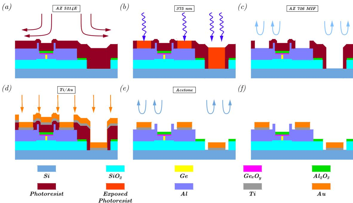
**Figure 3.6:** Depiction of the processing steps for the deposition of the Ti-Au reinforcement pads: (a) Spin-coating of AZ 5214E photoresist, (b) positive lithography step, (c) development of the photoresist, (d) sputter deposition of 10 nm of Ti and 180 nm of Au, (e) removal of excess material and residual photoresist using the lift-off technique, (f) completion of the process.
