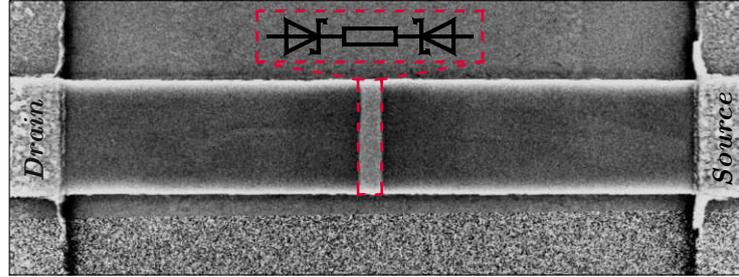
**Figure 2.14:** SEM image of a monolithic Al-Ge-Al heterostructure showing the drain and source contacts, along with an inset of the equivalent circuit diagram that features the back-to-back Schottky diodes and the channel resistance. Image based on [128].
