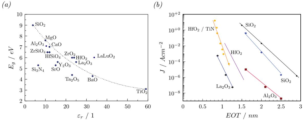
**Figure 2.4:** Important dielectric properties of potentially interesting high- $\kappa$  materials for the surface passivation of Ge. (a) depicts the band gap ( $E_g$ ) versus the relative permittivity ( $\epsilon_r$ ) lineup of different high- $\kappa$  materials. (b) indicates the measured leakage current density ( $J$ ) at 1 V for various high- $\kappa$  materials in dependence of the EOT. Image adapted from [85].
