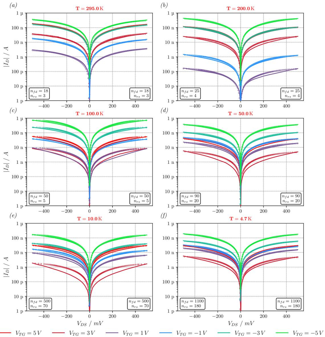
**Figure 4.7:** Semilogarithmic plot of the  $I$ - $V$  characteristics of device 03\_00 ( $l_{Ge} = 102 \mu\text{m}$ ) at various temperatures. The circles indicate the  $I$ - $V$  characteristics derived from the back-to-back Schottky diode device equation. Additionally, the fitting parameters related to the ideality factors are shown in the inset. Each subplot corresponds to a specific temperature at which the measurements were taken, ranging from 295 K down to 4.7 K. Image based on [132].
