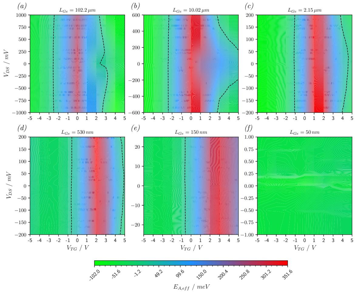
**Figure A.1:** Effective activation energy as a function of the gate and bias voltage for devices with Ge segment lengths of  $102 \mu\text{m}$  (a),  $10 \mu\text{m}$  (b),  $2 \mu\text{m}$  (c),  $0.5 \mu\text{m}$  (d),  $0.15 \mu\text{m}$  (e), and  $50 \text{ nm}$  (f). A dashed contour line indicates the value of  $k_B T$  at  $300 \text{ K}$ . Image based on [128].
