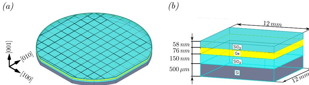
**Figure 3.1:** Structural layout sketch of the GOI wafer. (a) A 150 mm GOI wafer featuring sawn-out  $12 \times 12\ \text{mm}^2$  dies. (b) Dimensions of a  $12 \times 12\ \text{mm}^2$  GOI substrate, which includes a monocrystalline Ge device layer oriented in the  $\langle 100 \rangle$  direction, along with a BOX layer in between and a  $\text{SiO}_2$  capping layer on top. Image adapted from [149].
