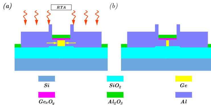
**Figure 3.5:** The formation of abrupt Al-Ge Schottky junctions through RTA: (a) The thermal out-diffusion of Ge into Al reservoirs results in a continuous movement of the Al-Ge interface along the Ge channel. (b) Final Al-Ge-Al heterostructure characterized by abrupt Al-Ge junctions and a controlled length of the Ge segment.
