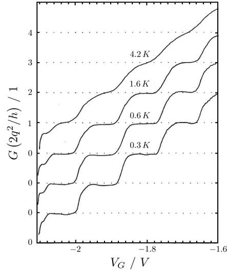
**Figure 2.17:** Quantization of conductance at temperatures of 0.3 K, 0.6 K, 1.3 K, and 4.2 K as a function of gate voltage in a GaAs/Al<sub>0.33</sub>Ga<sub>0.67</sub>As heterojunction. Image taken from [146].
