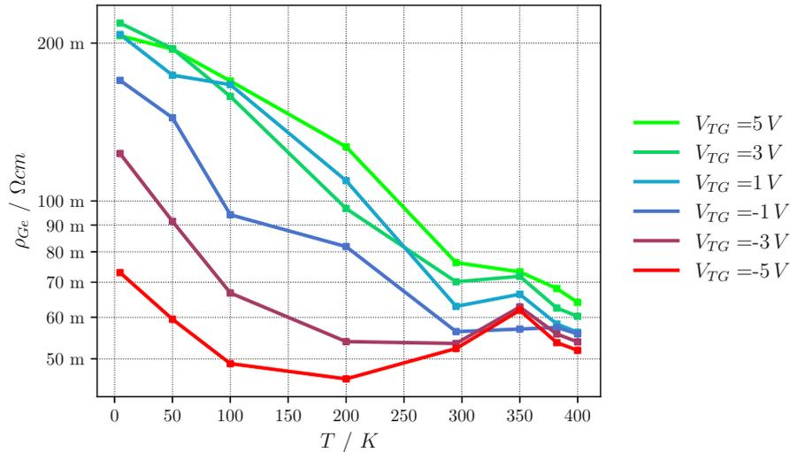
**Figure 4.22:** Device resistivity of device 08\_03 ( $l_{Ge} = 50 nm$ ) as a function of temperature and top-gate voltage calculated on the linear portion of the previously recorded I-V characteristics. The gate voltage ranges from  $-5 V$  to  $+5 V$ , with a voltage spacing of 2 V, while the temperature varies from 4.8 K to 400 K.  $\rho_{Ge}$  is presented in a logarithmic format.
