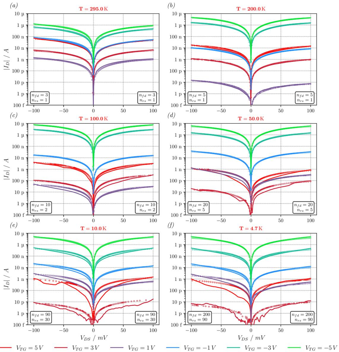
**Figure 4.12:** Semilogarithmic plot of the  $I$ - $V$  characteristics of device 11\_03 ( $l_{Ge} = 2 \mu\text{m}$ ) at various temperatures. The circles indicate the  $I$ - $V$  characteristics derived from the back-to-back Schottky diode device equation. Additionally, the fitting parameters related to the ideality factors are shown in the inset. Each subplot corresponds to a specific temperature at which the measurements were taken, ranging from 295 K down to 4.7 K. Image based on [132].
