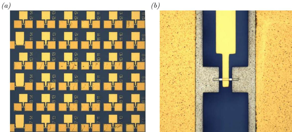
**Figure 4.2:** Images of the finished sample obtained through optical microscopy. Image (a) displays a section of the sample surface, while (b) presents an enlarged view of a channel section within the device.
