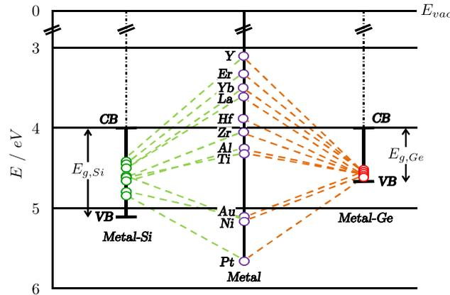
**Figure 2.12:** Illustration of the Fermi-level pinning for Si and Ge. The work function of various metals is shown along with the band gap of Si and Ge, referenced to the vacuum energy level  $E_{vac}$ . The dashed lines indicate the pinning of the metal's Fermi level in Si and Ge, respectively, when they are brought into contact. As demonstrated, the red dashed lines representing the metal-Ge contact are all pinned close to the valence band (VB). Image adapted from [122, 123].
