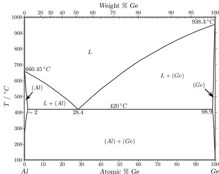
**Figure 2.5:** Phase diagram of the eutectic Al-Ge system. The melting points are given as  $660^\circ\text{C}$  for Al and  $938^\circ\text{C}$  for Ge. The eutectic point is found at  $420^\circ\text{C}$  and 28.4% (at) Ge. The maximum solubility of Al in Ge is 2% (at) and Ge in Al is 1.1% (at). [36, 100] Image adapted from [101].
