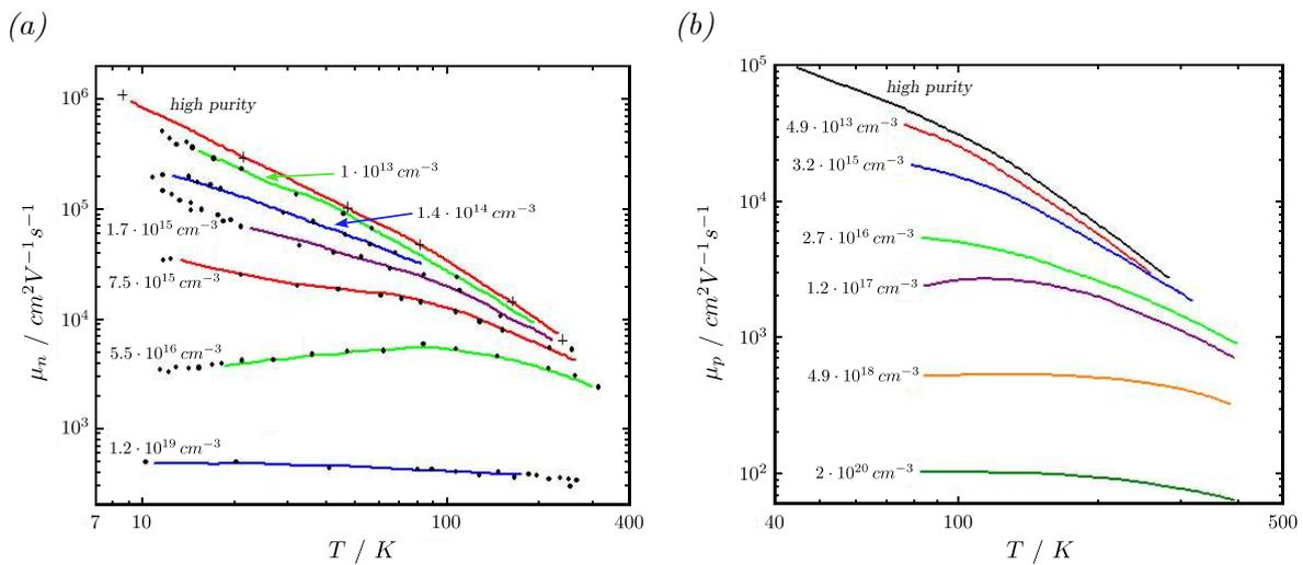
**Figure 2.3:** Minority carrier mobility of electrons (a) and holes (b) as a function of temperature and doping concentration  $N_A - N_D$ . The mobilities of the high-purity Ge in subfigures (a) and (b) were measured using the time-of-flight technique. [73] The mobilities of the doped Ge were determined via the Hall effect. [74, 75] Image adapted from [76].
