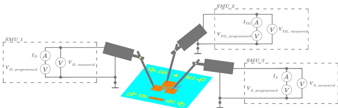
**Figure 3.8:** Schematic representation of the connections for the drain, source, and gate, along with a basic circuit diagram of the SMUs. A Keysight B1500A semiconductor analyzer is used to carry out the electrical characterization with the help of three SMUs, which are connected via triaxial cables to the needle probes.
