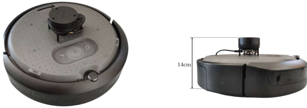
(a) Robot Platform with mounting plate (b) Side-view to outline setup height
