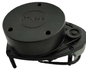
Figure 3.2: Slamtec LiDAR sensor RPLIDAR A1M8
