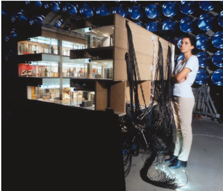
Fig. 2 Model of shopping mall (scale 1 : 20 / artificial sky).
