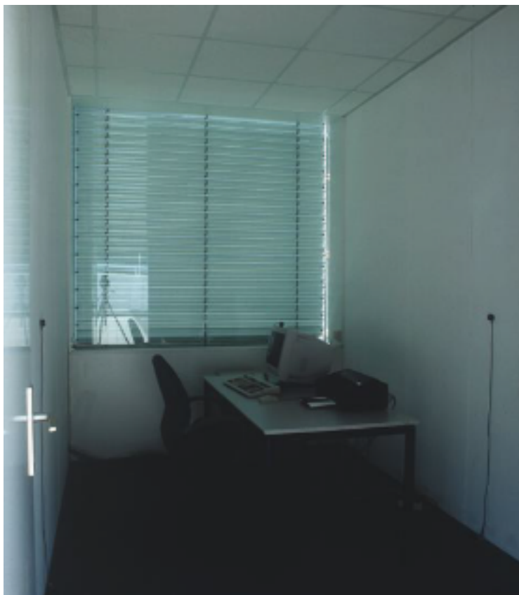
Fig. 6 Office with conventional blind outside (no daylight inside the room).
