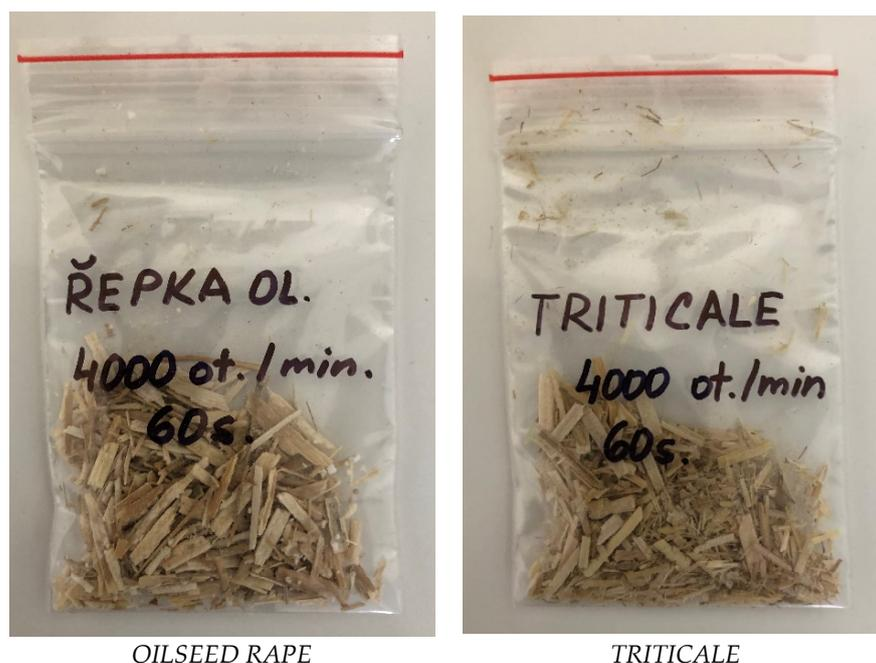
**Figure 5.** Test samples of straw pulped at 4000 rpm and a grinding time of 60 s.
