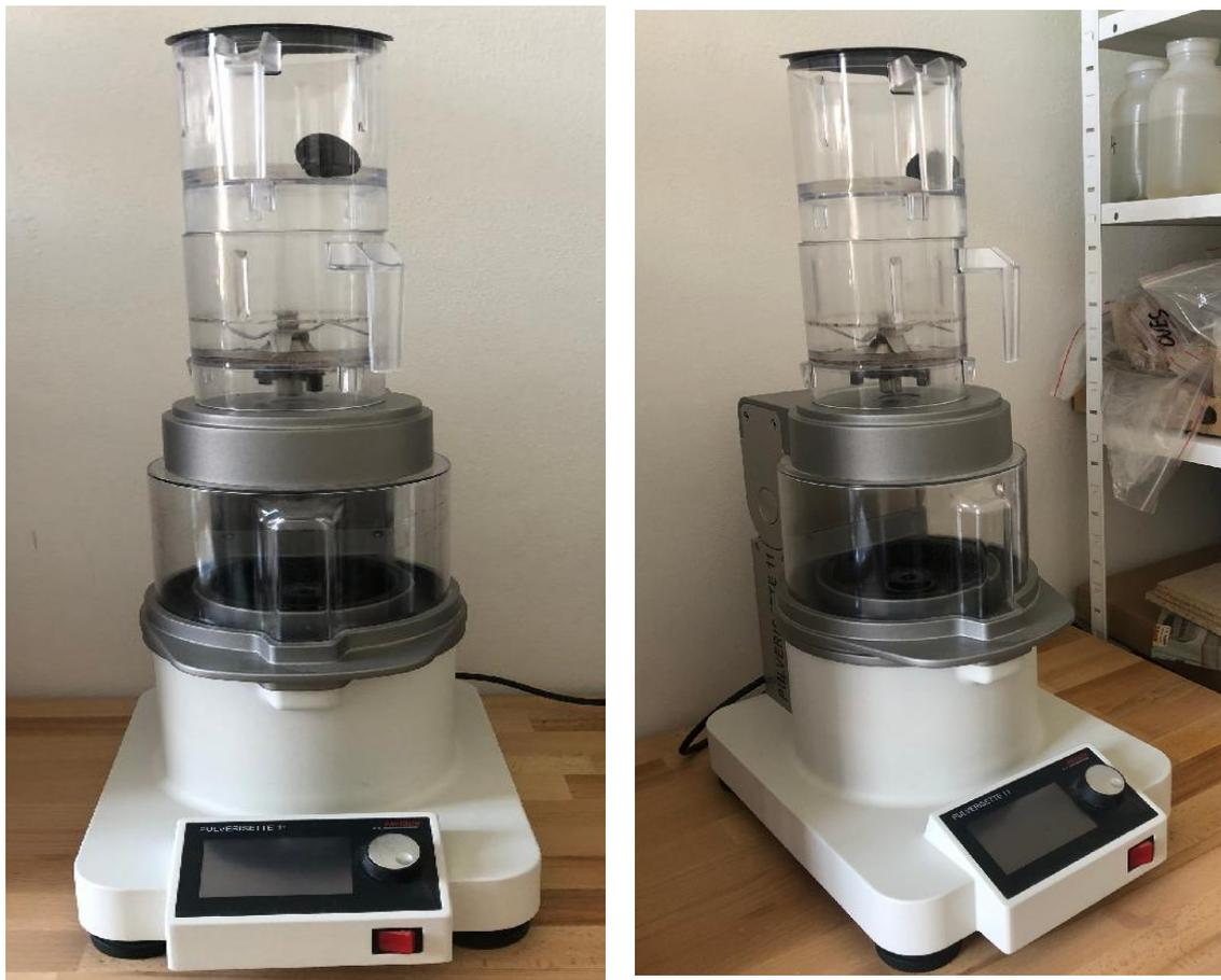
**Figure 4.** Knife mill Pulverisette (FRITSCH, Weimar, Germany).
