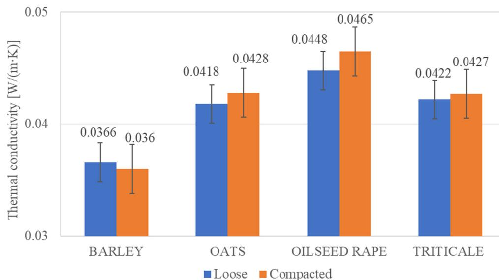
**Figure 14.** Comparison of thermal conductivities of free-flowing and compacted samples (mechanically pulverized at 4000 rpm and a grinding time of 60 s).
