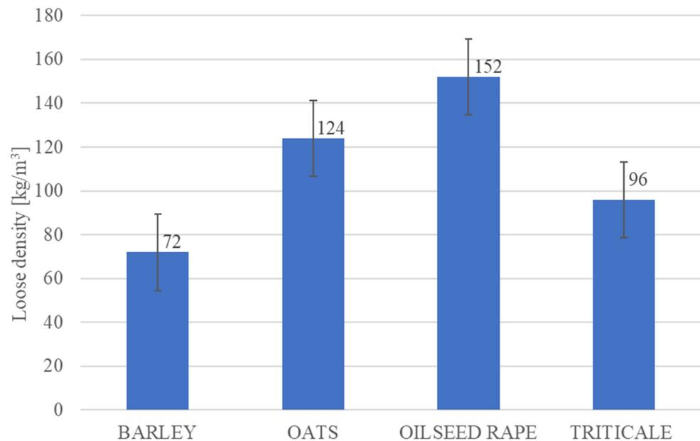
**Figure 6.** Comparison of bulk weights of individual straw samples pulped at 4000 rpm and grinding time of 60 s.
