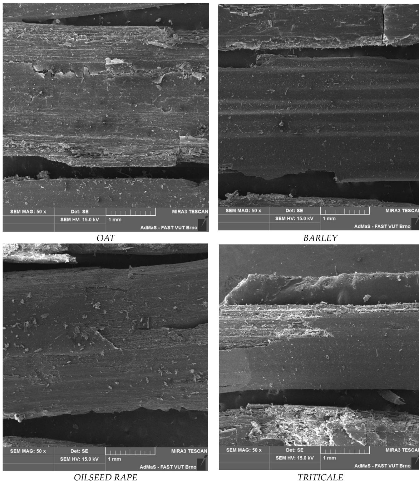
**Figure 3.** Images of straw from electron microscope TESCAN MIRA3 XM (Brno, Czech Republic), magnification 50 $\times$ .
