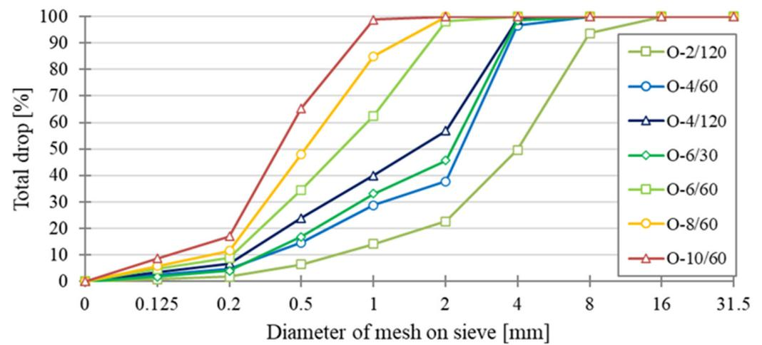
Figure 8. Sieve analysis of oat samples.
