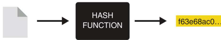
Figure 3.5: Exemplary workings of a hash function [100].
