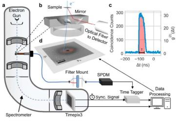
Experimental Setup: (a) Collected photons and transmitted electrons are detected in a time resolved manner. (b) A sample holder equipped with ellipsoidal mirrors is used to collect CL photons. Electrons and photons are coincidence matched according to their time difference, which is shown as a histogram in (c). The low angle diffraction pattern (d) for the coincidence-matched electrons (in red) differs significantly from the unmatched image (in grayscale).
