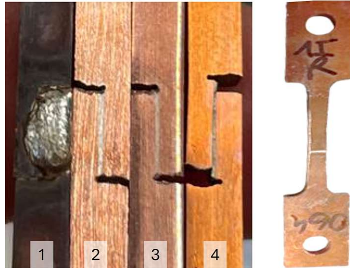
Figure 22: Progress of the solder joint preparation for the stress-relaxation-tests.
