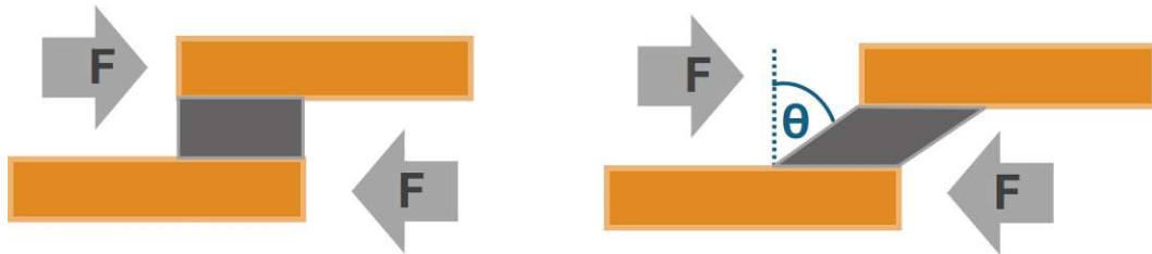
Figure 10: Scheme of a shear test with lap-shears joints.
