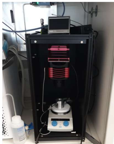
Figure 4.2. Pictures of POM gas-phase reactor prototype (a) and reaction setup installed into a black box (b).
