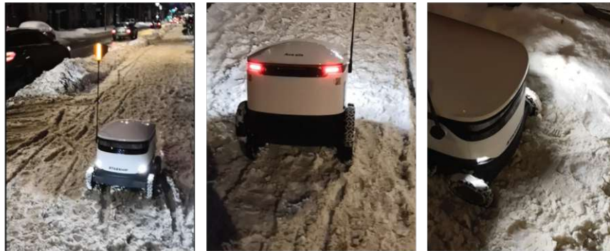
Figure 4.7: Three images depicting different angles on the same scene – a Starship robot is trying to free itself out of heavy snow by lifting its wheels. December 2021.
