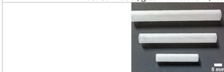
Fig. 2: Tubular PCL-scaffolds, manufactured by 3 D printing (MEW/FDM).
