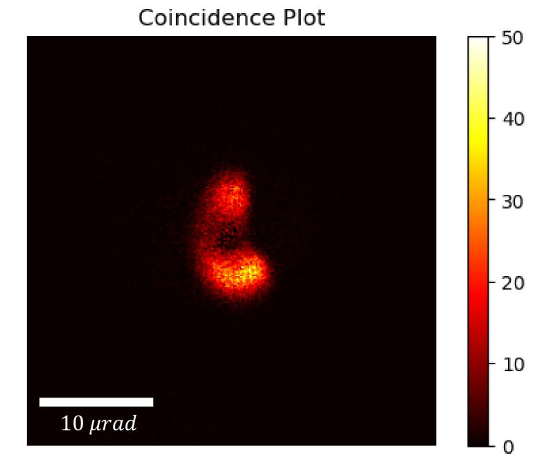
Although electrons don't directly interact with the mirror, in the presented coincidence plot we are able to observe a ghost image of the parabolic mirror and even small features such as the beamhole with a size of 300  $\mu m$ .
