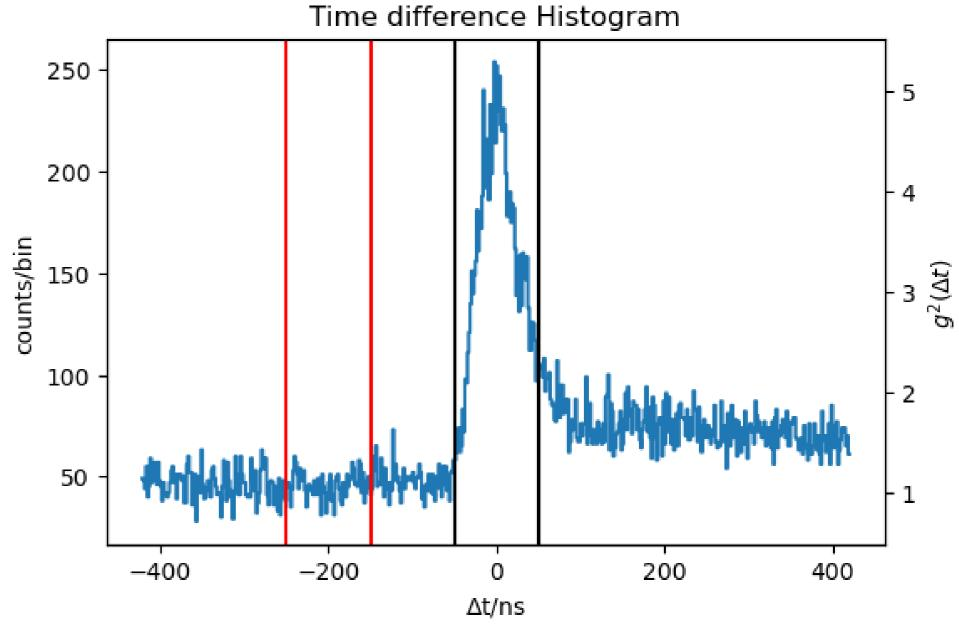
The resulting coincident histogram has a full width at half maximum (FWHM) of 80 ns. Black bounds represent electron-photon coincidences, red bounds correspond to background coincidences. To improve SNR we subtract background coincidences from real signal. The following plot is obtained by capturing correlated electrons with the Timepi3 camera.
