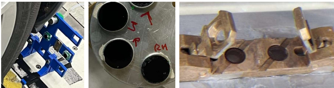
Fig 1: Collection of tire abrasion particles behind the rear tire in the lab on the test bench.
