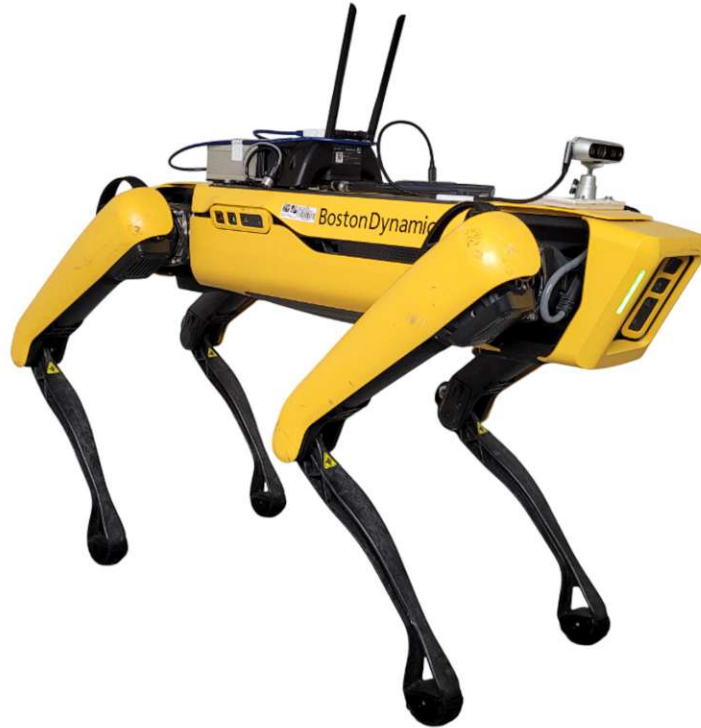
(a) Boston Dynamics Spot robot equipped with Spot Core and a depth camera.
