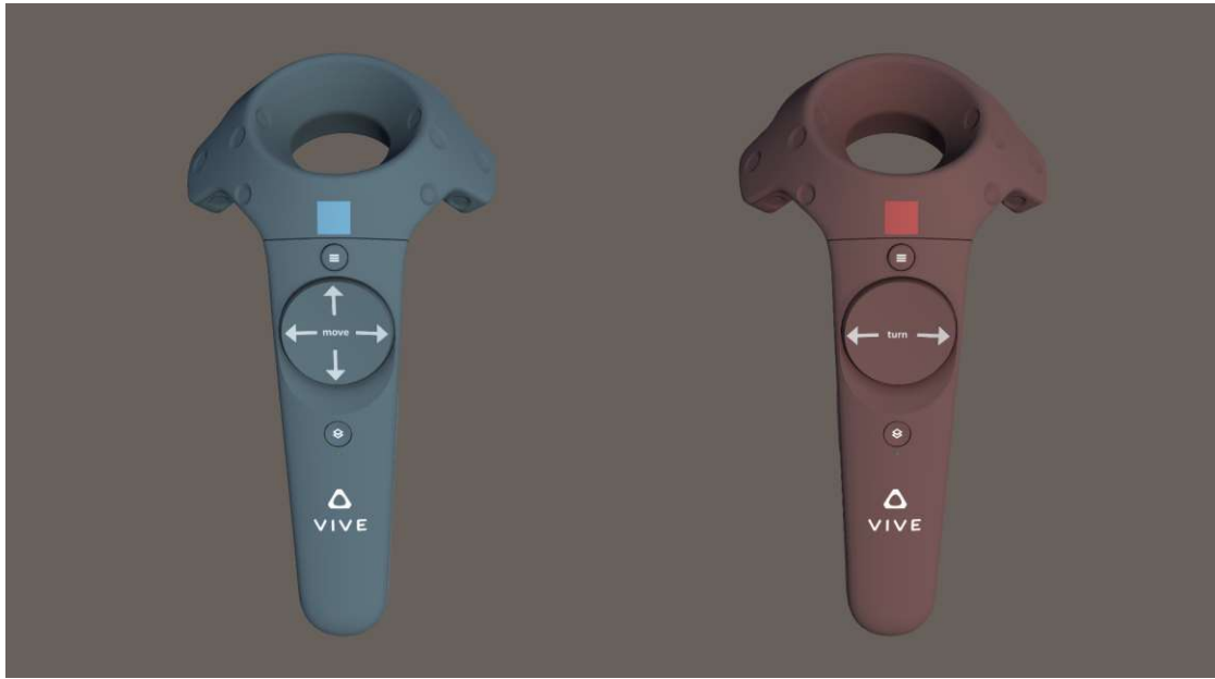
Figure 3.12: Virtual controllers for direct control of the mobile robot. Left controller: handles linear movement to move forward, backward and to the left and right. Right controller: responsible for rotational motion to turn left and right.
