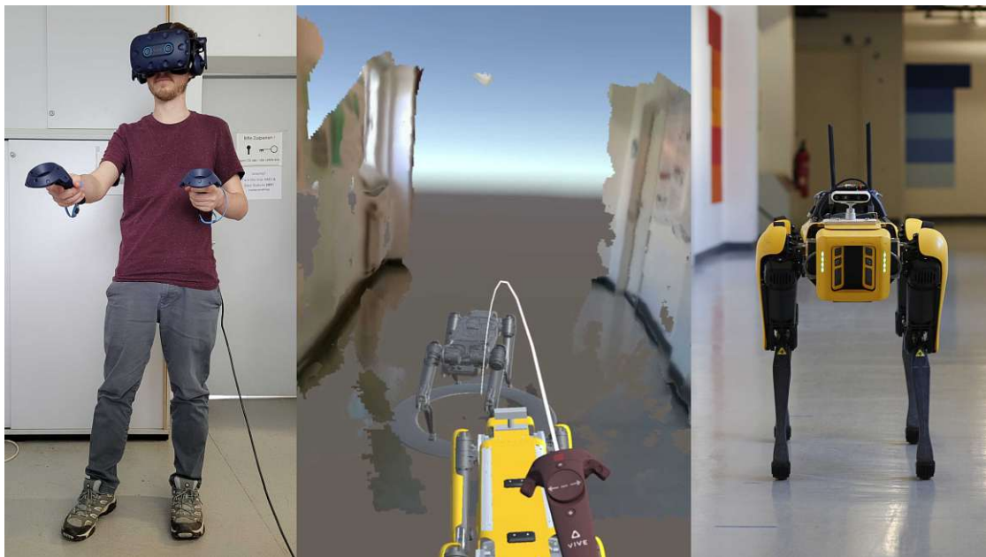
Figure 4.2: Image compilation of the user study execution. Left: User in the test room with the VR headset on and the VR controllers in hand. Middle: User view of robot and the Point-and-Click navigation metaphor in the reconstructed environment. Right: Physical robot in the hallway.
