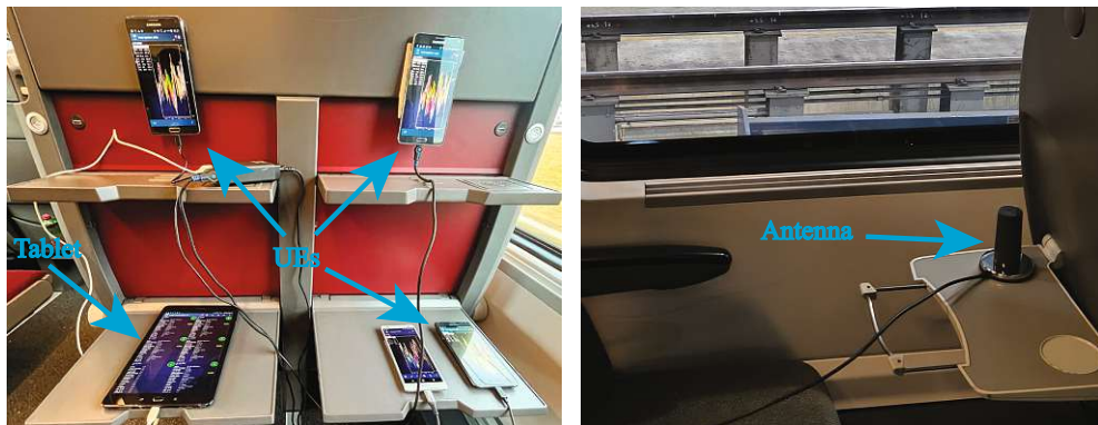
Figure 2.7: Measurement setup for indoor train testing. On the left side, a tablet acts as the master unit, automatically triggering measurement scripts on all connected UEs . On the right side, an external antenna is positioned as an alternative setup option and used for scanner-based measurements (though the scanner itself is not visible in the image).
