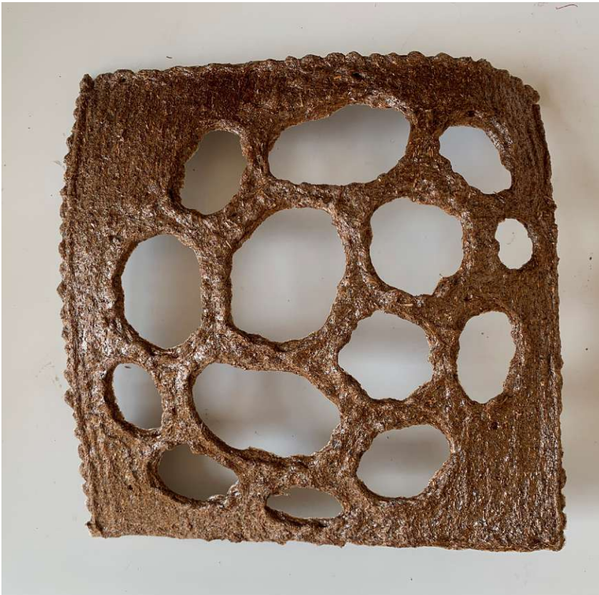
prototype 2. mixture 13 + 7,7% wood flour. dry
