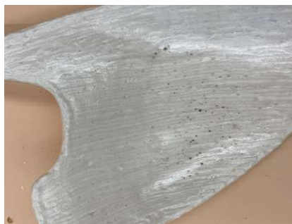
mould appeared during drying time
