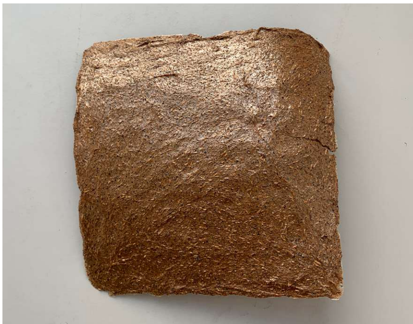
casted mixture 13 + 7,7% wood flour, dry
