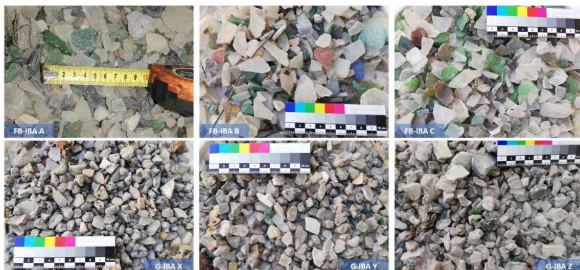
Fig. 3. Sensor-based separated glass-fractions 8–35 mm from incineration bottom ashes from fluidized bed (top) and from grate (bottom).
