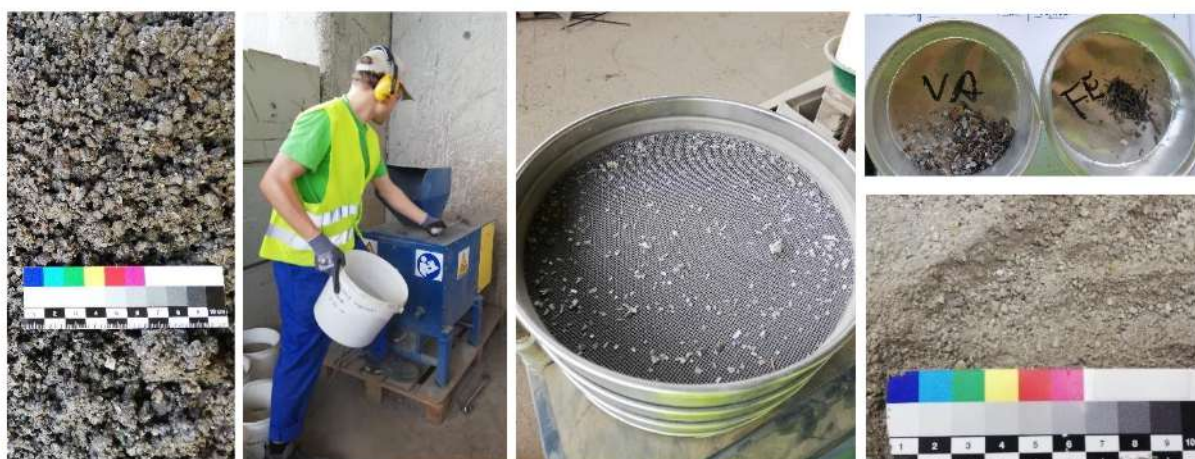
Figure 8: Determination of residual metal pieces, from left to right: mineral fraction <8 mm, crushing of the mineral fraction, sieving of the crushed material, metals after crushing (top) and crushed mineral material (bottom)
