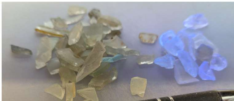
Figure 7: Fluorescence of lead glass on the right side when exposed to UV-C light
