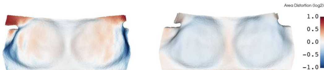
Figure 5.12: Comparison of flattening approaches: Preserving individual arc lengths (left), Using the middle contour for uniform scaling (right).
