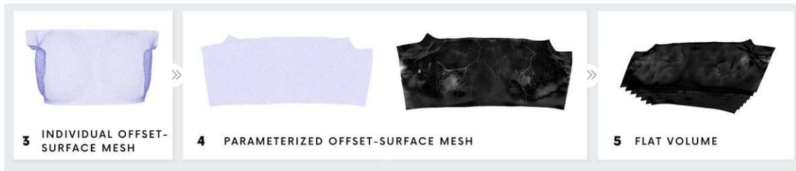
Figure 5.3: Overview surface cutting approach: Each surface is individually flattened using ARAP parameterization (4), then aligned and stacked to reconstruct a volumetric representation (5).
