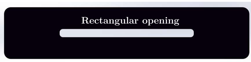
Figure 3.14: The rectangular aperture mask for creating a strip of light with a 2.5 mm opening.
