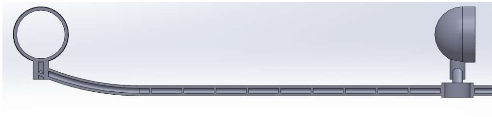
Figure 3.9: Sectional view of an arm and a paddle. The arm has a partially hollow structure.
