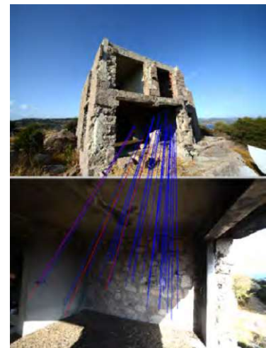
Figure 5.9: Example of tie points established between one outdoor photo of Building 1 and one photo taken from the inside.
