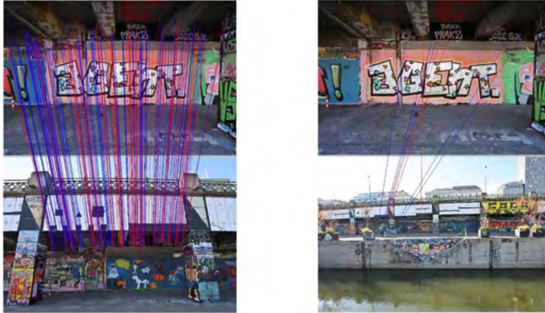
Figure 4.7: Example of valid tie points (blue lines) established between one image of a new graffiti (Upper; 17 December 2021) and two images covering the same site but 52 days earlier and with significant differences in texture. The two lower photos were acquired during the full photographic coverage on 27 October 2021. Adopted from [53].
