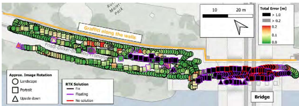
Figure 4.14: Camera positions with colour-coded total positional error. The south-east portion of the map shows photos taken beneath the steel bridge. Camera symbols represent their orientations, while the border colours indicate the RTK solution status. The wall of interest with graffiti is marked by the orange line on the northern side. Adopted from [57].
