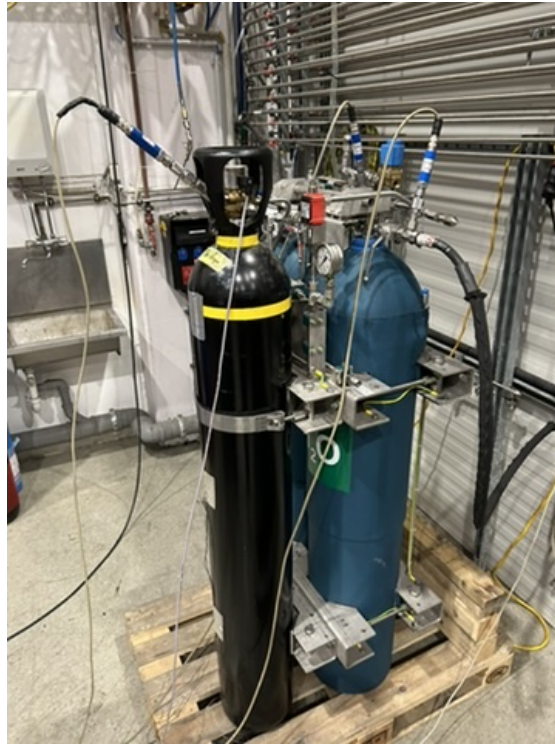
Figure 5.1: Gas vessel (black) and water vessel (blue) mounted in a GPP fixture. The three blue cylinders connected to the gray cables are HySense PR 400 piezoelectric pressure sensors.
