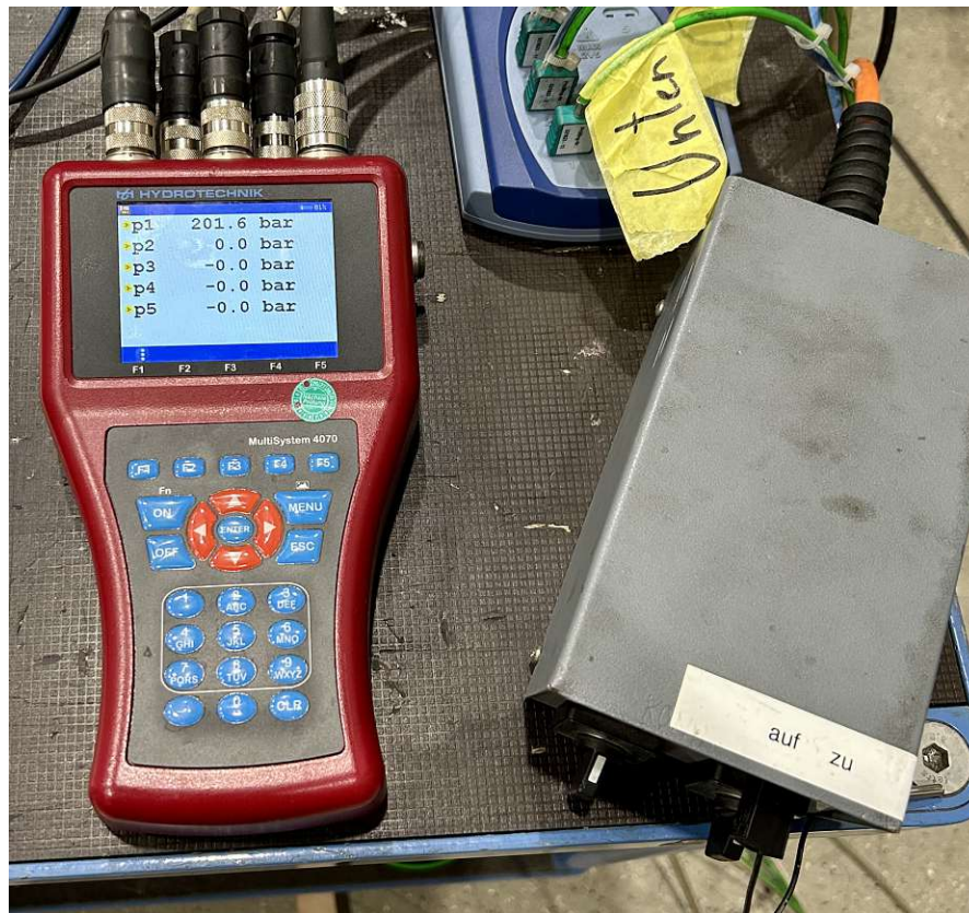
Figure 5.4: Multisystem 4070 used for recording the pressure measurement values. The gray box on the right is the manual trigger for the trigger valve to open. At the time when this picture was taken, the valve was still closed, as can be seen on the multisystem where the gas vessel pressure is at the initial pressure of 202 bar while all other pressures are zero.
