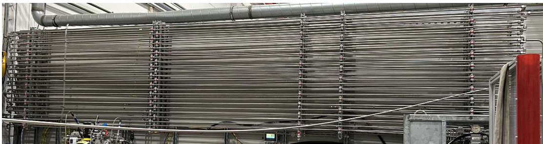
Figure 5.2: Piping system to simulate a real life situation where the water has to flow through long pipes to reach the nozzle head.
