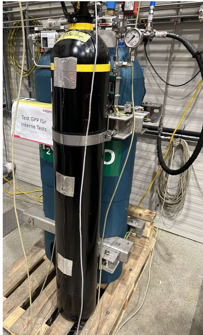
Figure 5.5: Type K thermocouples were attached to the gas vessel at three different positions using self-adhesive and thermally insulating aluminum foil.
