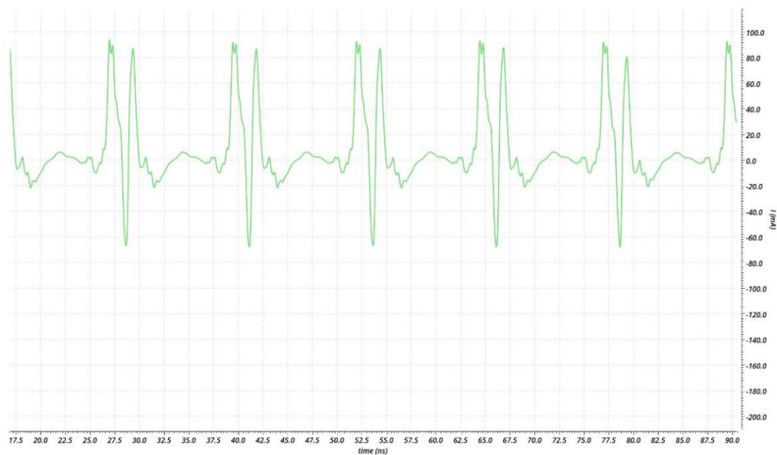
Figure 102: Post-layout simulation of 4.05V supply current (external Gater).
