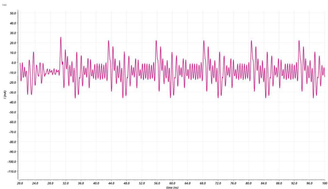
Figure 111: Post-layout simulation of 6.6V supply current (PWM ASIC)
